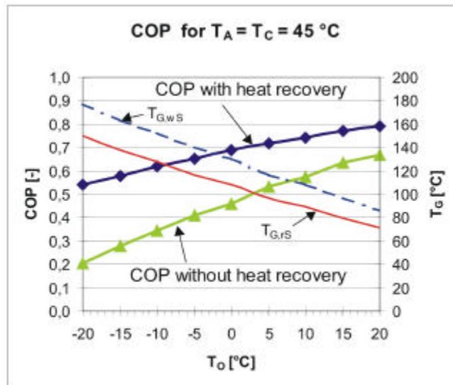
**Figure 2:** Coefficient of performances (COP) of the DACM with/without heat recovery for evaporator temperatures from  $-20$  up to  $+20^\circ\text{C}$  and for  $T_A = T_C = 45^\circ\text{C}$  (simulations).
