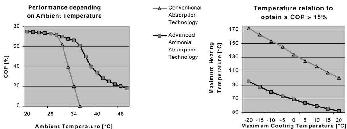
Figure 2: Low Temperature Absorption Chiller versus Conventional Absorption Chiller – Performance Indicators
