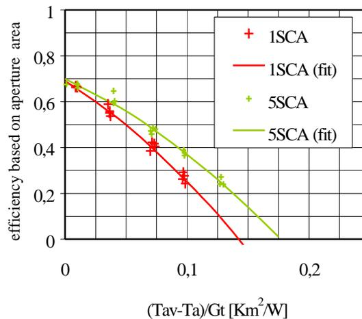
Steady state efficiency curves of two of the stagnation proof transparently insulated collector prototypes (called 1SCA and 5SCA, for use up to 90°C and 120°C respectively).
