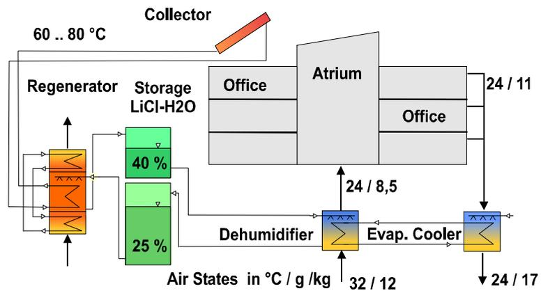
Figure 2. Solar air dehumidification and storage system
