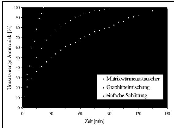
Characteristic of the matrix heat exchanger
