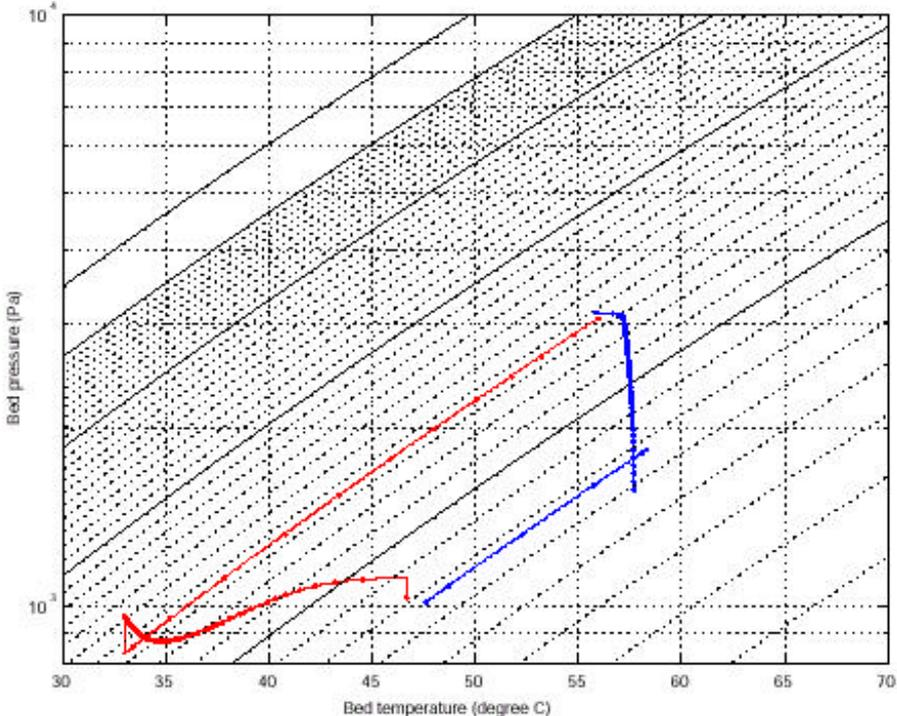
Figure 4 Duehring diagram of the cycle-steady -state condition of the beds.
