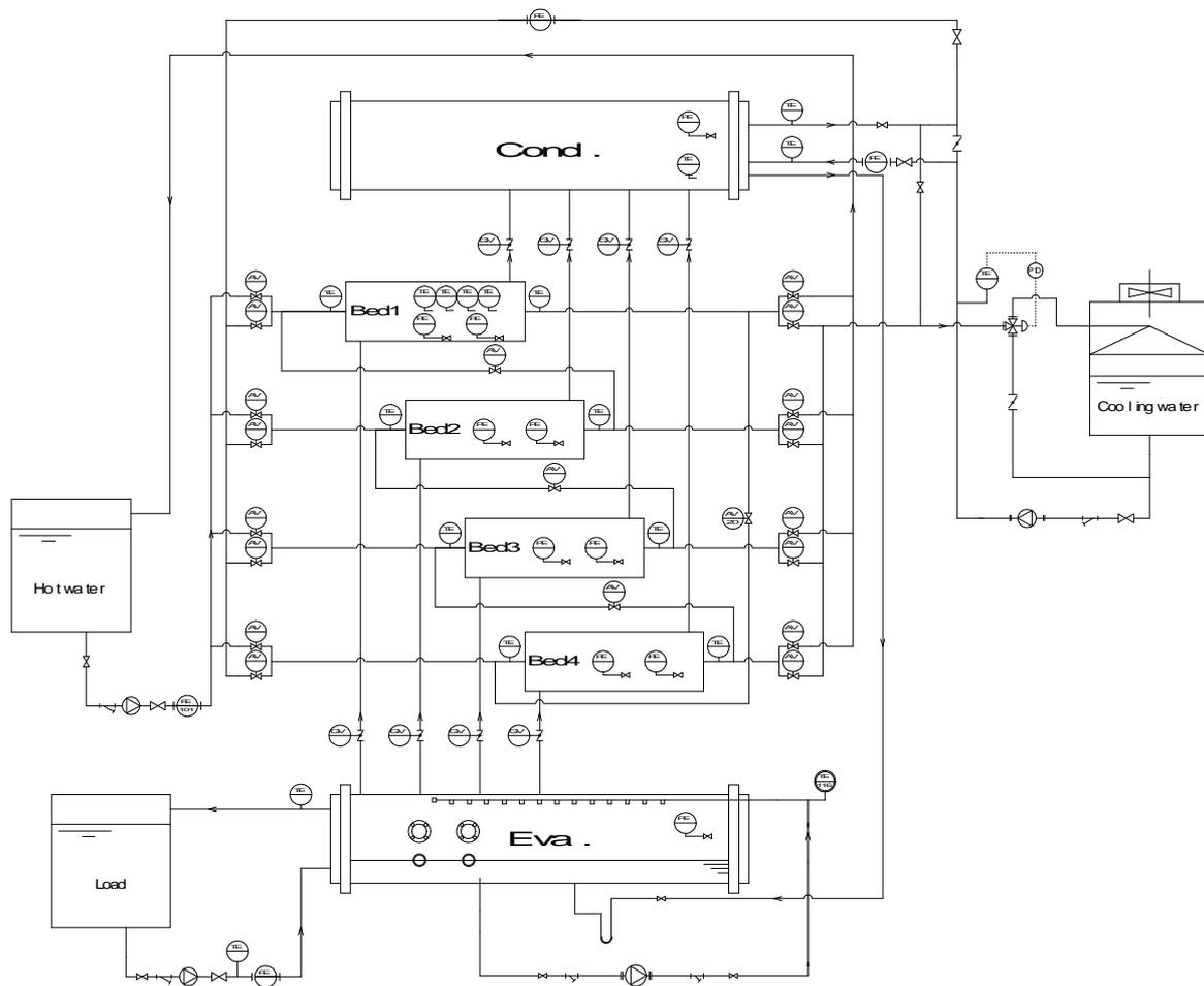
Figure 1: Schematic flow diagram of a 4-bed chiller
