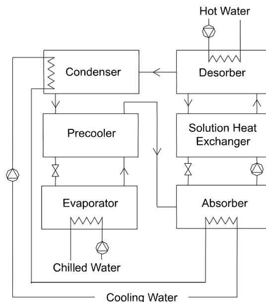
As shown the prototype is a simple effect absorption machine.
