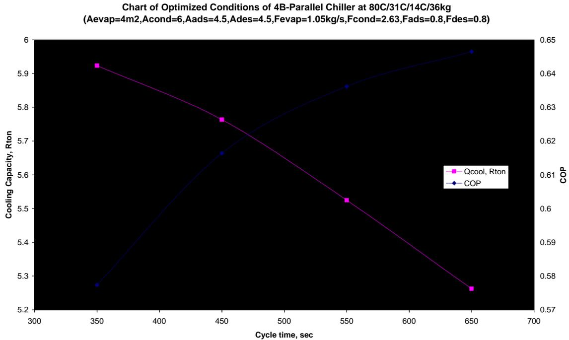
Figure 2: Cooling capacity and COP as a function of cycle time
