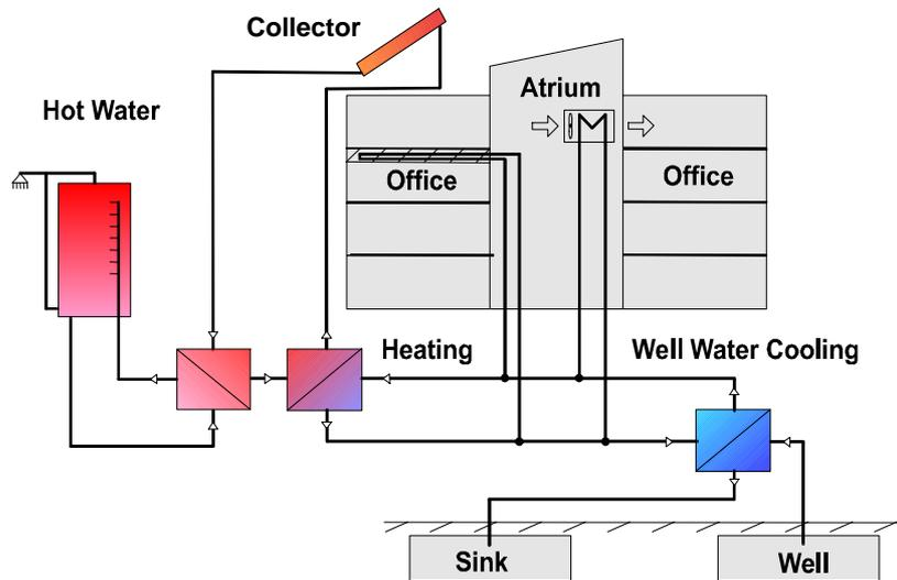
Figure 1: Structure cooling and heating. Solar hot water and optional solar space heating.
