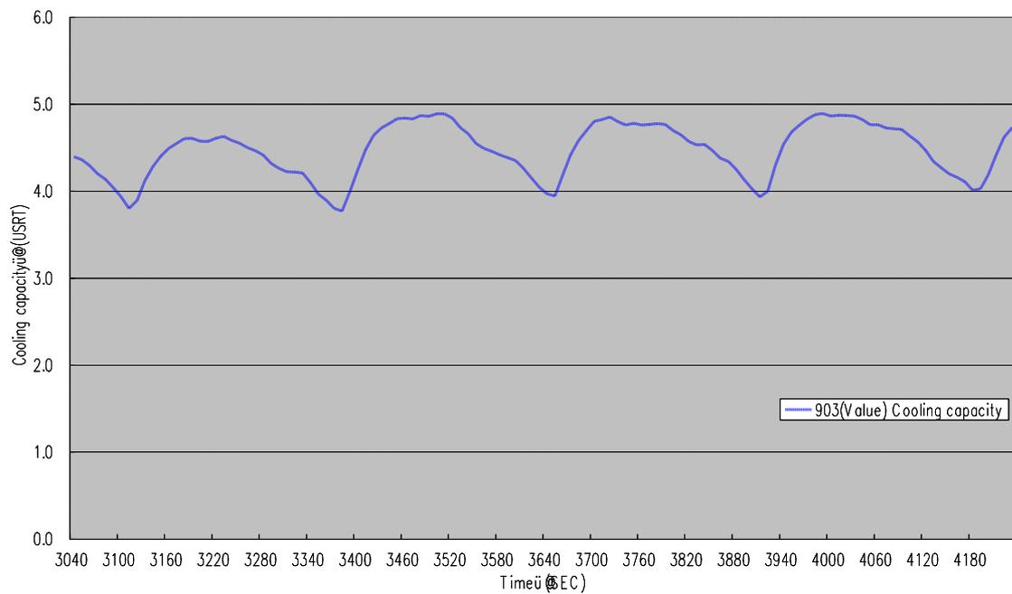
Figure 3: Cooling capacity profile of a 4-bed adsorption chiller
