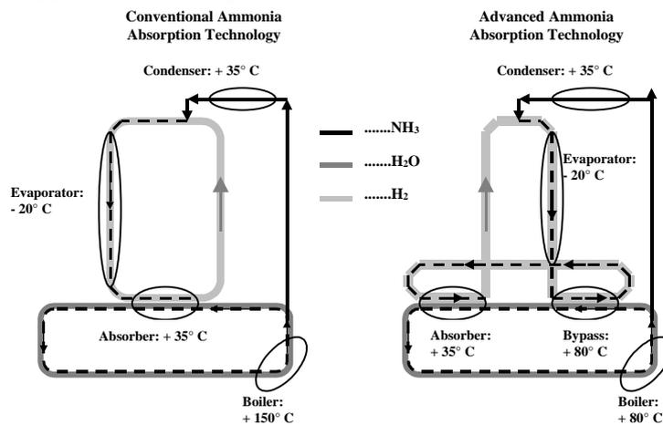
Figure 1: Advanced (Low Temperature) Ammonia Absorption Chiller versus conventional ammonia diffusion absorption chiller – Schematic
