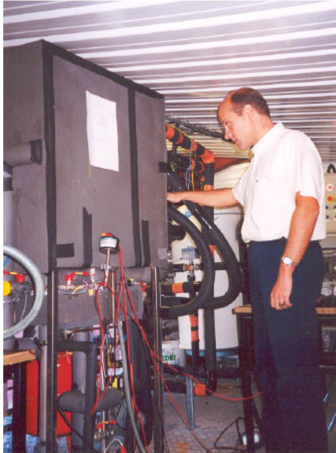
***Prototype absorption heat pump***
