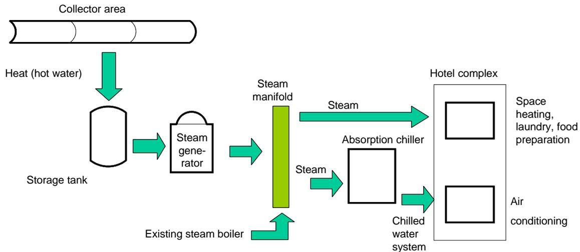
Thermal energy flows in absorption air conditioning system operated through solar energy and supply with steam boiler
