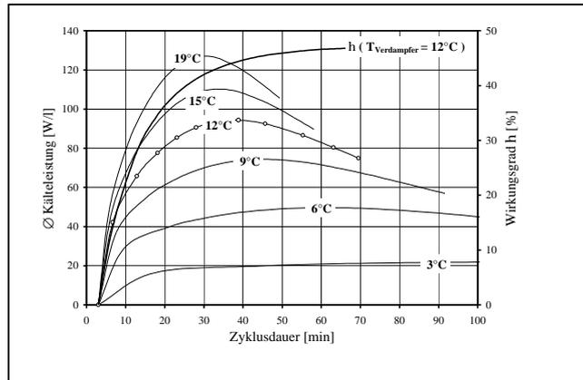
Dependence of average cooling capacity from evaporator temperature and cycle time
