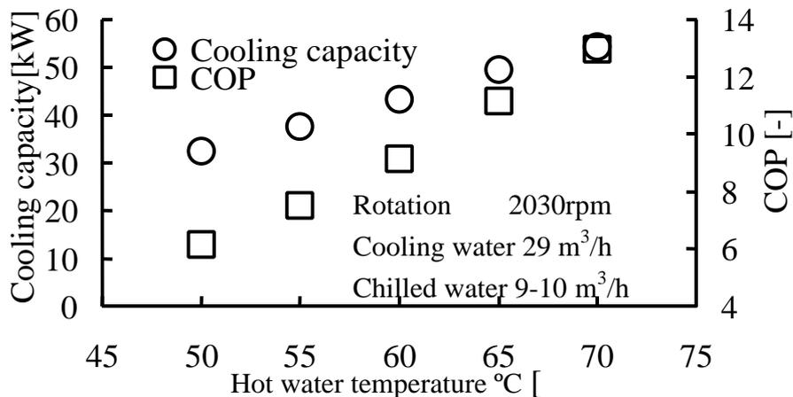
Fig.5 Hot water temp. dependency on cooling capacity & COP
