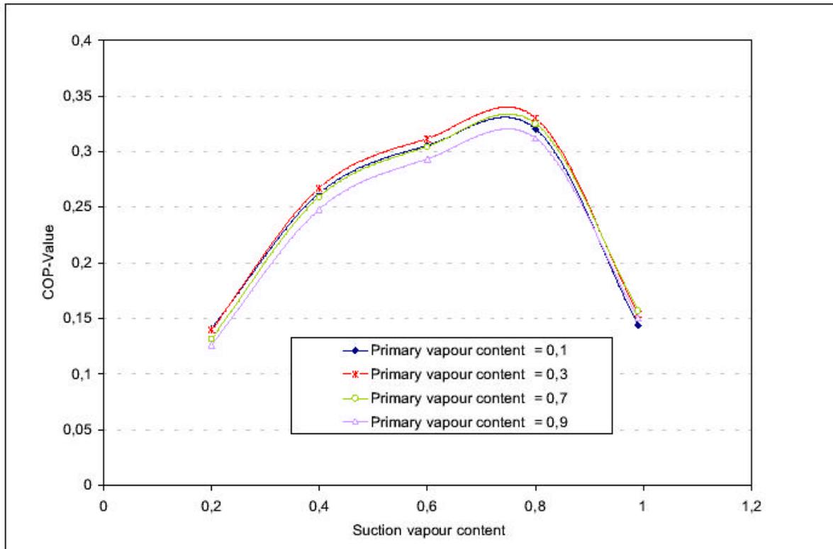
Figure 3: COP versus vapour content of the secondary flow, on suction side of the ejector, at various vapour contents of the primary flow for a composition of 99% ammonia and a mixing section efficiency of  $\eta_M = 0.7$  (the mixing section is part of the ejector).
