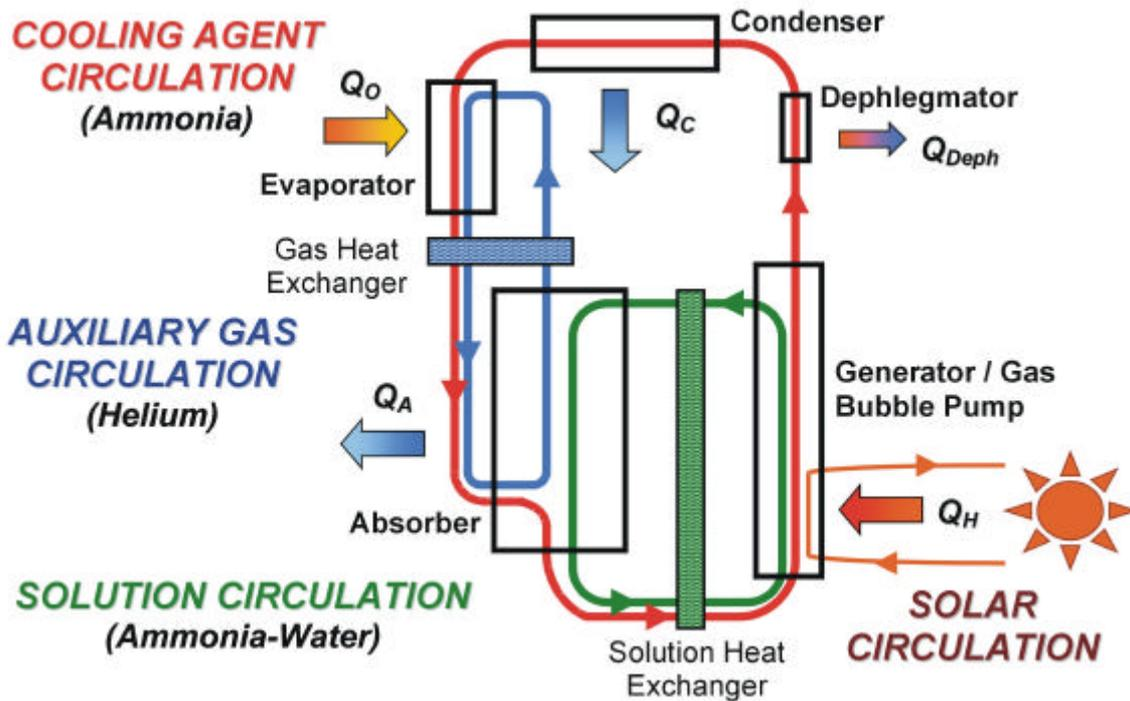
**Figure 1:** Principle of the solar driven Diffusion-Absorption Cooling Machine (DACM).
