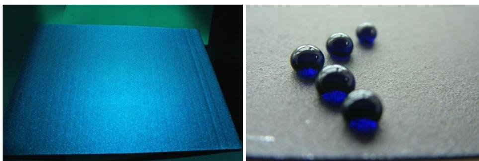
Colored TISS coating on PPS absorber (left) and colored water droplets on TISS paint surface (right).
