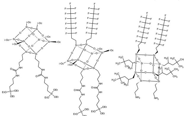
POSS molecules proposed as an additive for decreasing free surface energy of TISS coatings.
