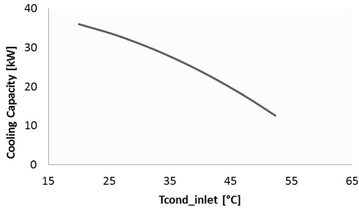
Figure 6 Part loads vs. the inlet temperature at the condenser
