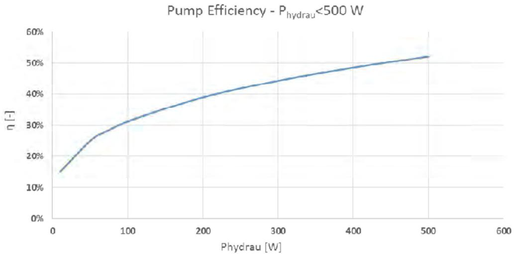
**Figure 3 Pump efficiency vs. its hydraulic power (<500W)**
