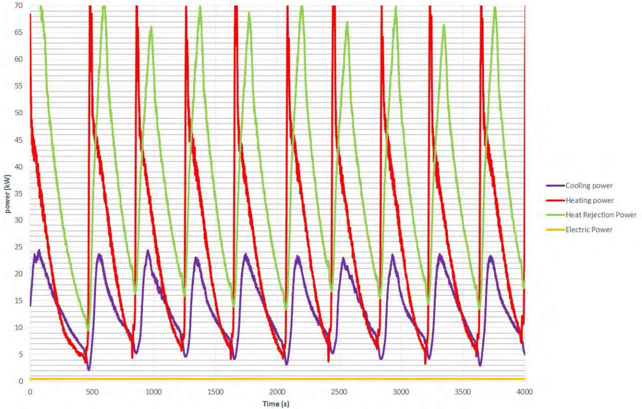
**Figure 11: power trends for a test with low condensation temperature.**
