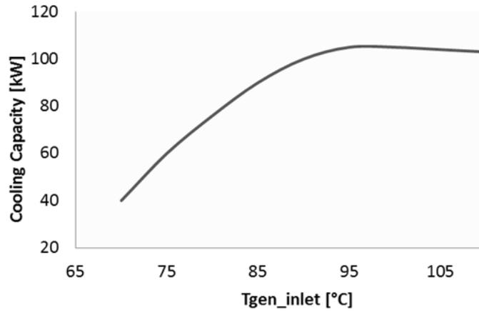
Figure 5 Part loads vs. the inlet temperature at the generator
