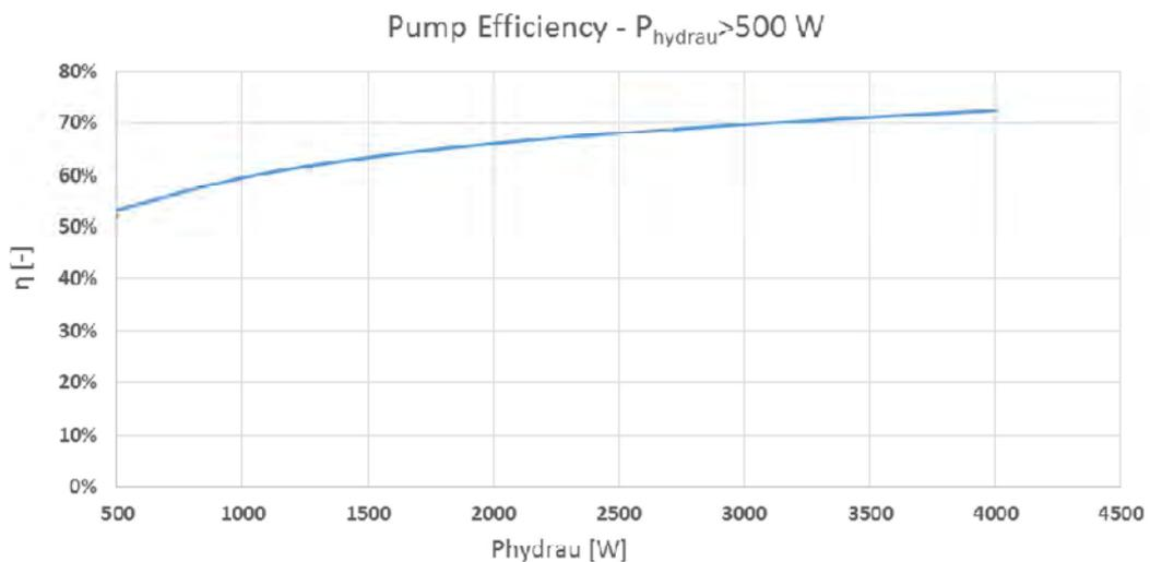
**Figure 4 Pump efficiency vs. its hydraulic power (>500W)**
