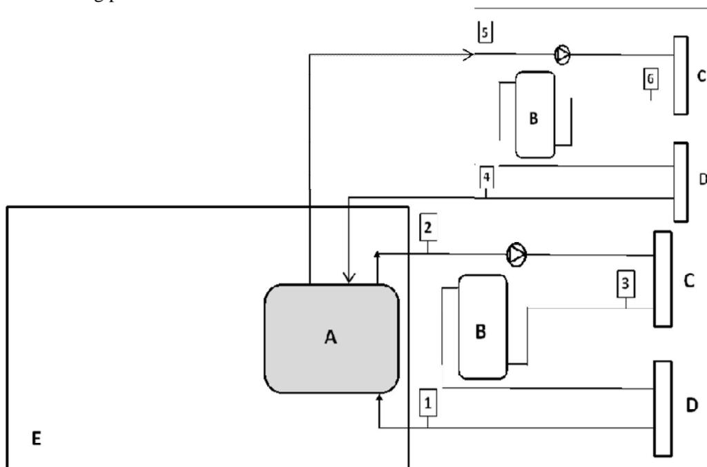
**Figure 8 Compensation systems for air-to-water/brine chillers**
