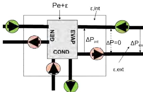
Figure 2 System boundary used for the definition of Test Methods and performance evaluation procedures
