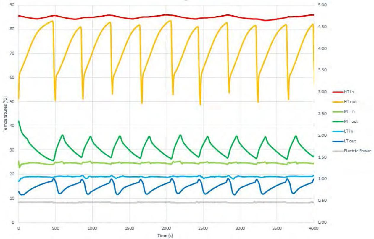
**Figure 10: temperature trends for a test with low condensation temperature.**
