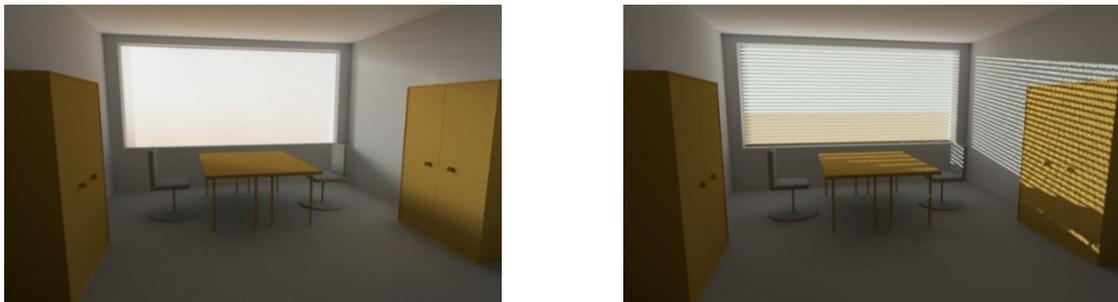
**Figure 12:** Simulation of a daylighting system represented by its BSDF (left) and by a combination of BSDF and geometry (right)
