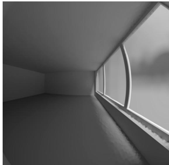
**Figure 40:** Daylight distribution for double clear glass rendered with Radiance
