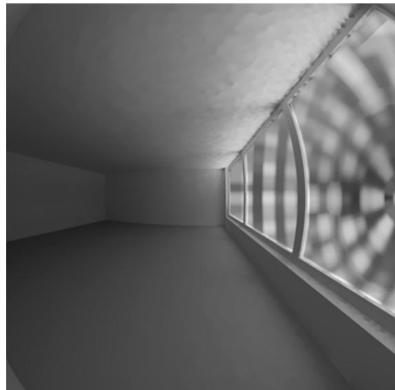
**Figure 49:** Daylight distribution for lasercut panel rendered with Radiance
