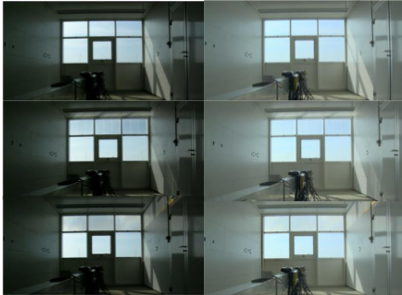
**Figure 2:** Interior view of daylight modules DEMONA equipped with different complex fenestration systems on the upper part of the façade : (top) standard insulating glazing, (centre) laser cut panel and (bottom) 3M SOLF prismatic film; left and right images have different exposure times.
