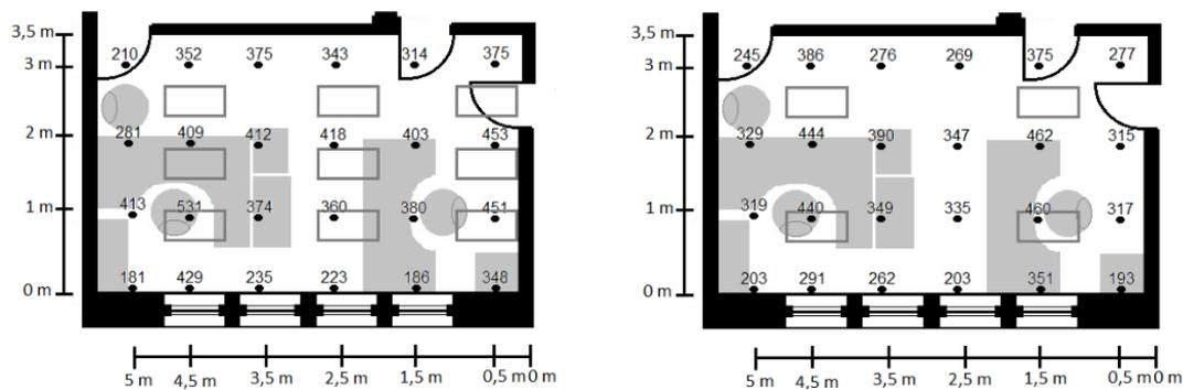
Figure 1: Illuminance distribution from electric lighting system pre- and post-retrofit (right) situations in office s.238 at Horsens Town Hall, Denmark.
