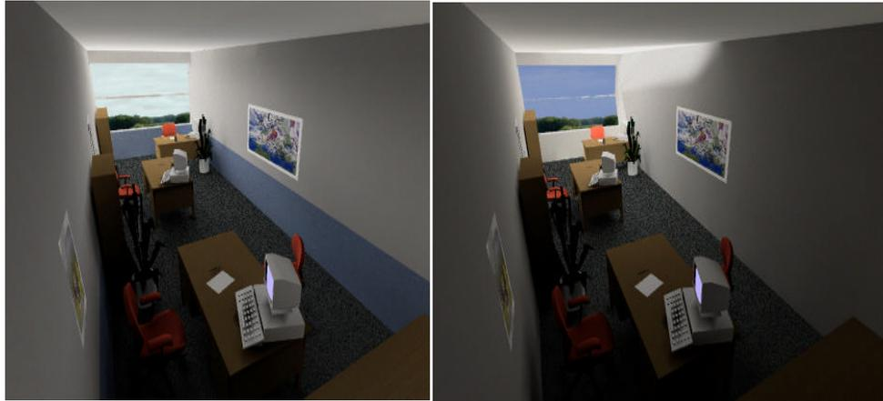
Fig. 11 Daylighting simulation of simple glazing (left) and Serraglaze (right) – Opposite views.
