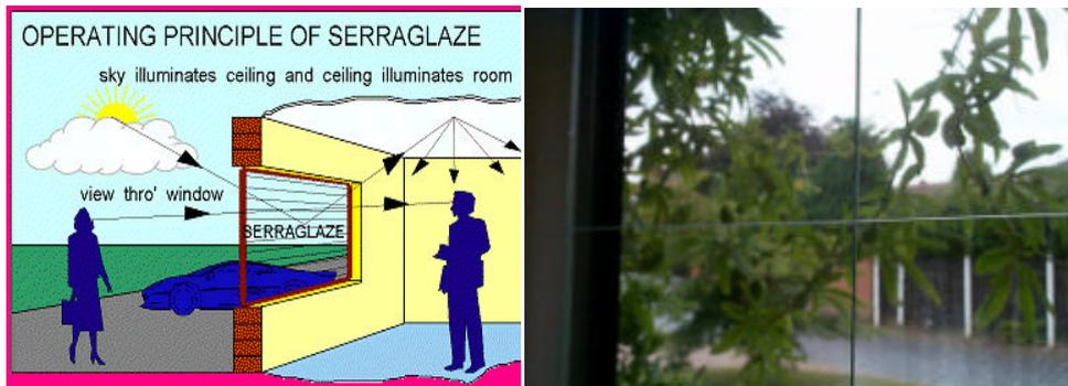
Fig. 4 Operating principle of the Serraglaze product (left), and view through the window (right).
