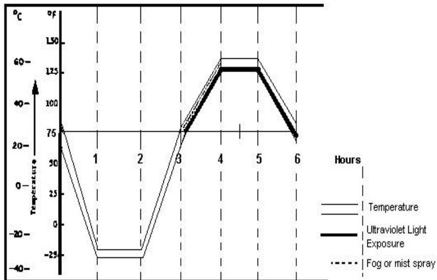
Note-This figure represents the ideal cycle described in this test method. Any temperature variation within the tolerance zone shown is acceptable.
