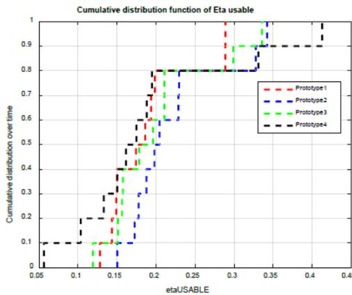
FIG. 13  $\eta_{usable}$  cumulative frequency distribution for Adaptiwall prototypes
