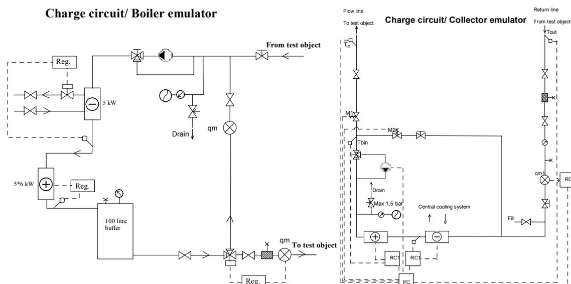
Figure 3: Charge module 1 at SP: auxiliary heating emulator.
