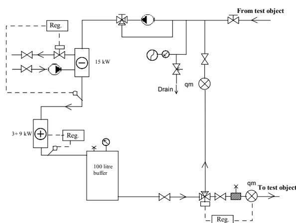
Figure 5: Discharge module.
