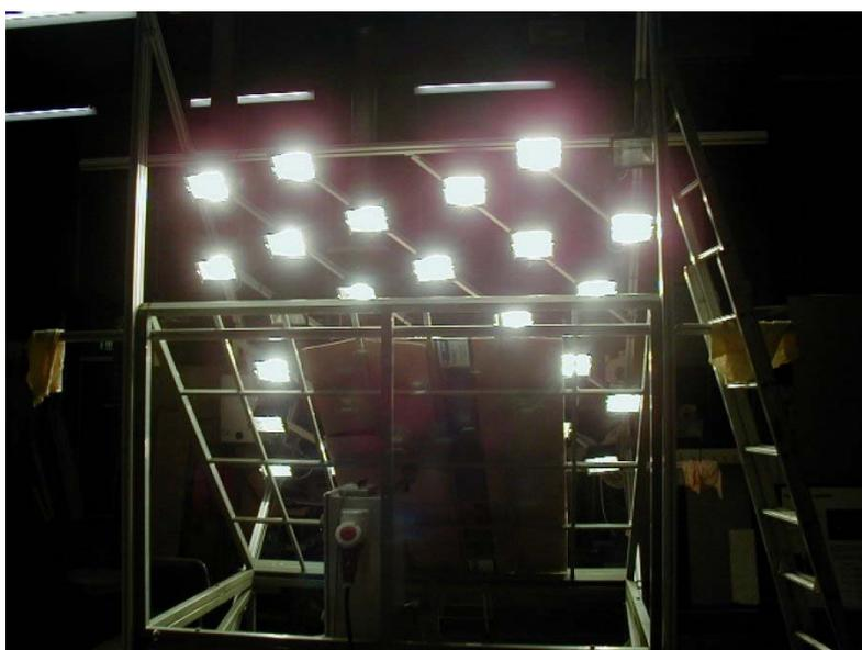
Figure 8: The solar simulator as part of the TNO test facility for solar combisystems.
