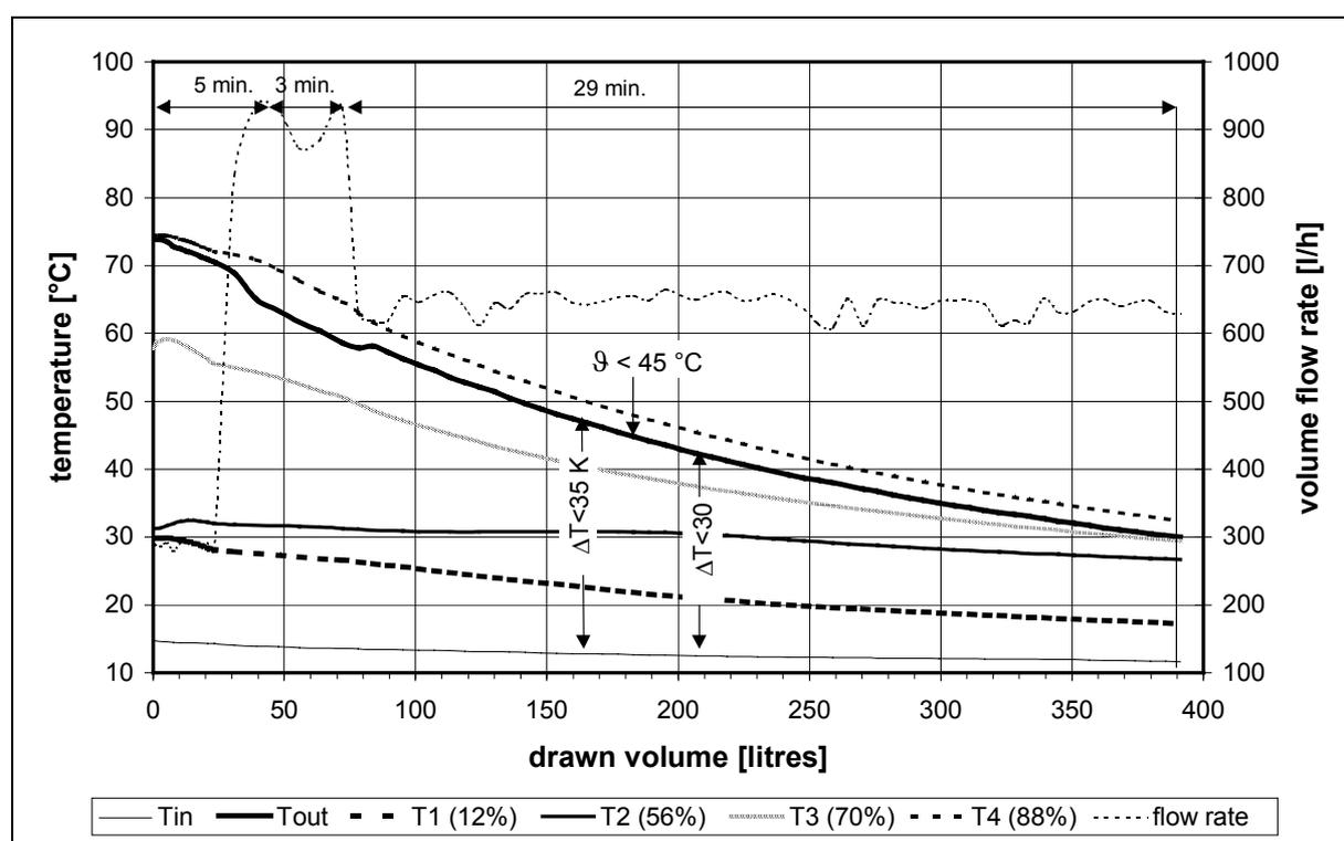
Figure 4.1: Temperatures and volume flow rate of store A (draw-off profile 300/900/600 l/h)
