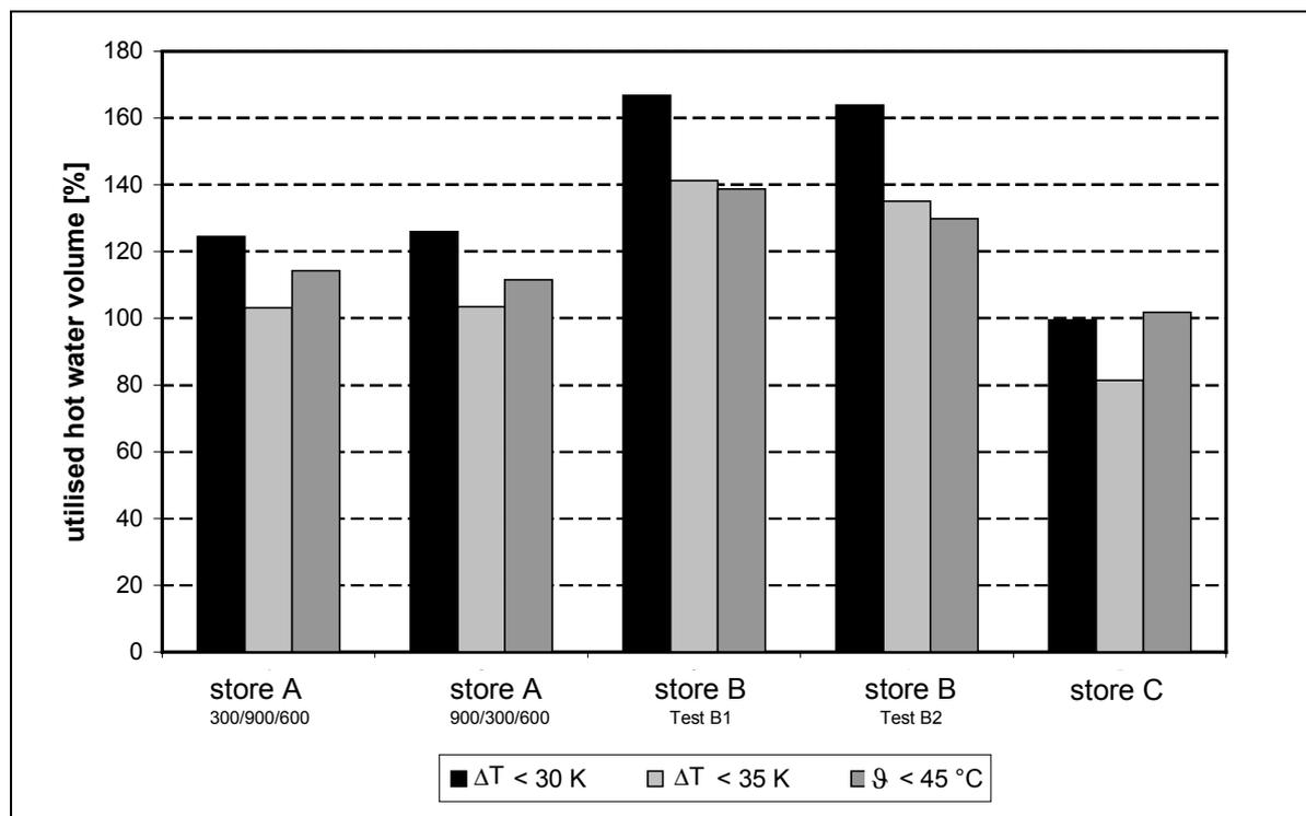
Figure 5.1: Utilised hot water volumes in percent (100 % correspond to 200 litres) determined for different termination criteria and draw off-profiles.
