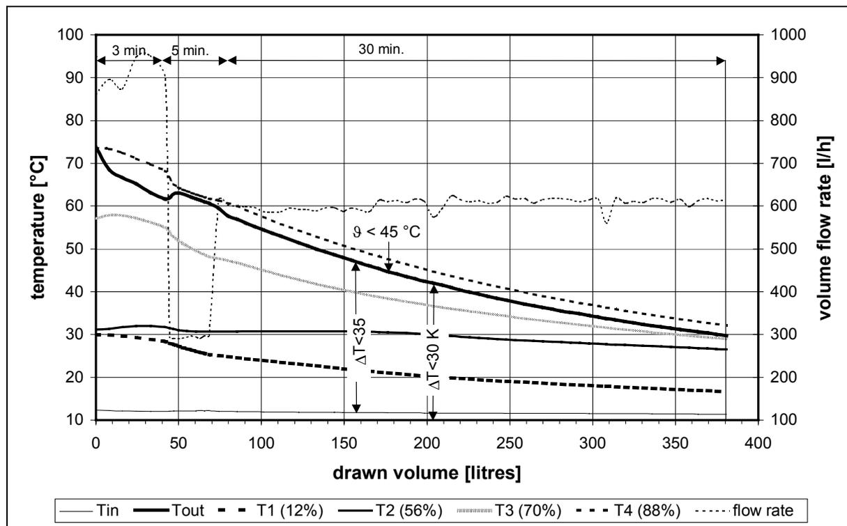
Figure 4.2: Temperatures and volume flow rate of store A (draw-off profile 900/300/600 l/h)
