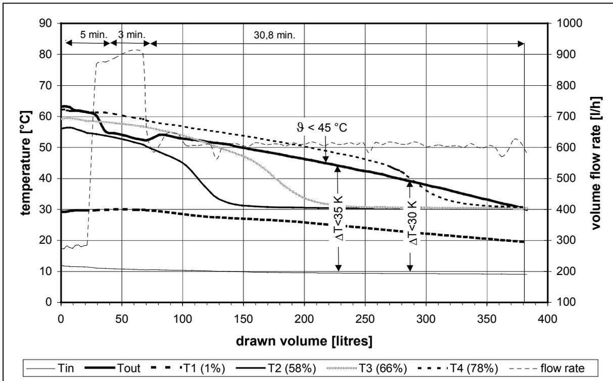
Figure 4.4:Temp. and vol. flow rate of store B (Test B2) (draw-off profile 300/900/600 l/h)
