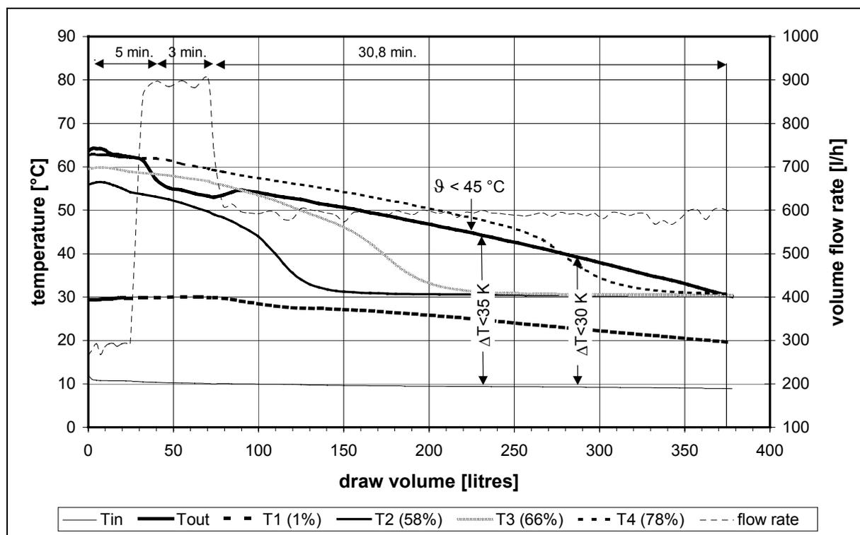
Figure 4.3: Temp. and vol. flow rate of store B (Test B1) (draw-off profile 300/900/600 l/h)
