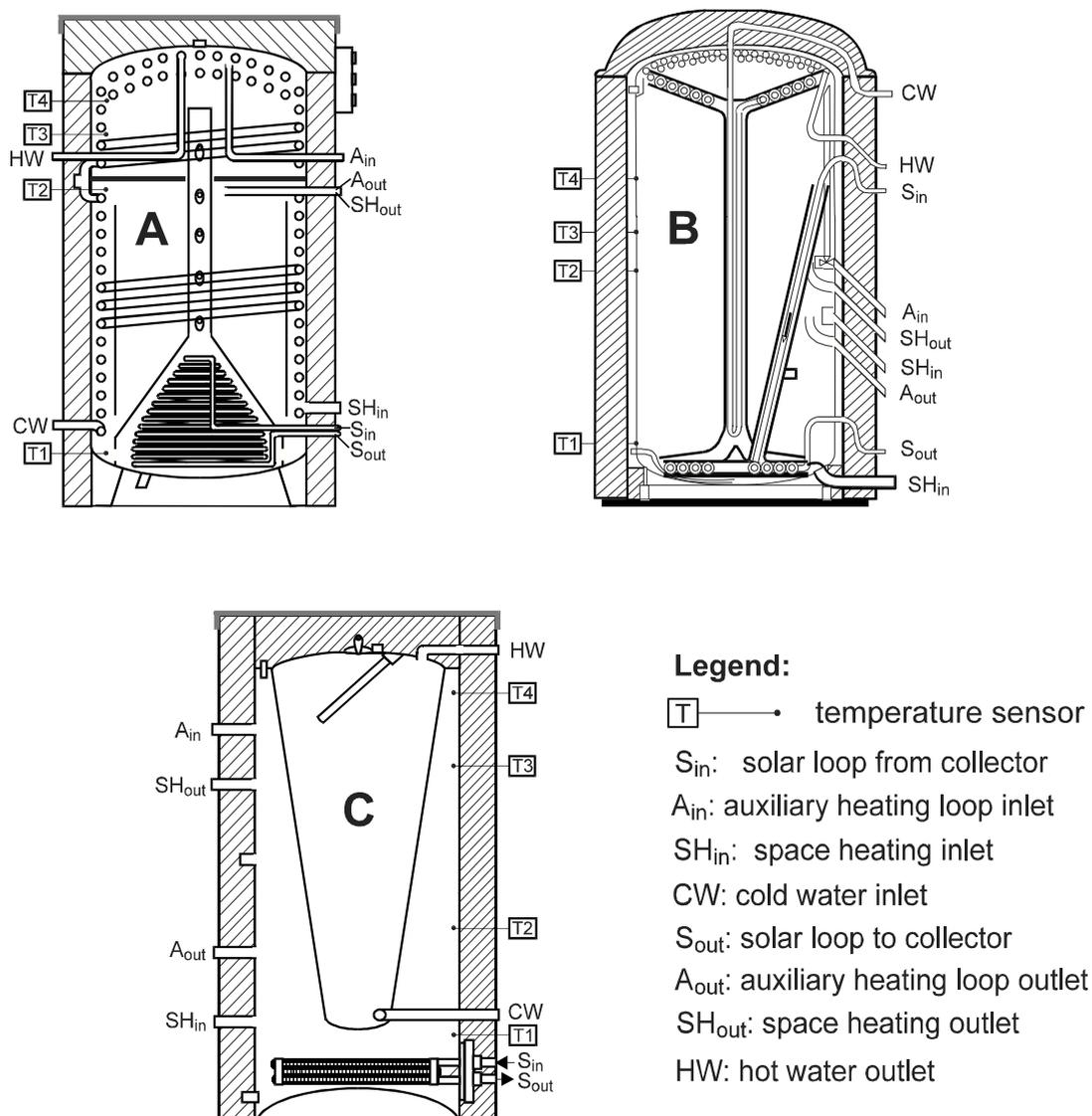
*Figure 1: Schematic setup of the three combistores*
