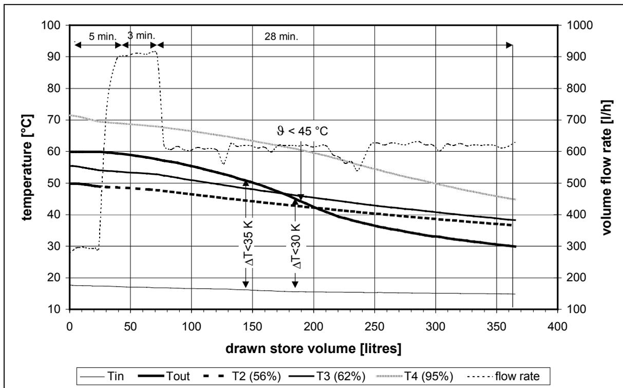
Figure 4.5:Temp. and volume flow rate of store C (draw-off profile 300/900/600 l/h)
