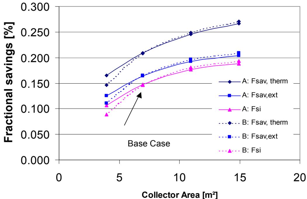
Figure 6: Control strategy A: Boiler running all year, B: Electric immersion heater used in summer
