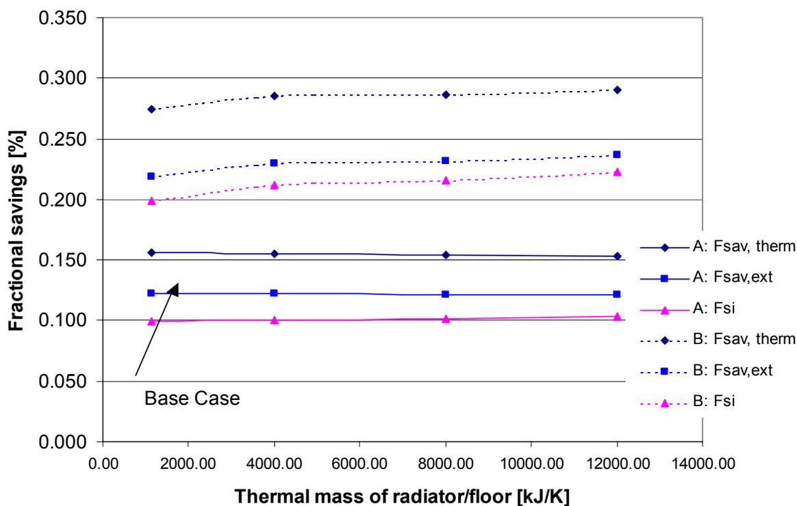
Figure 13: Variation of Radiator Thermal mass. A: 5 m<sup>2</sup> Solar Collector B: 15 m<sup>2</sup> solar collector
