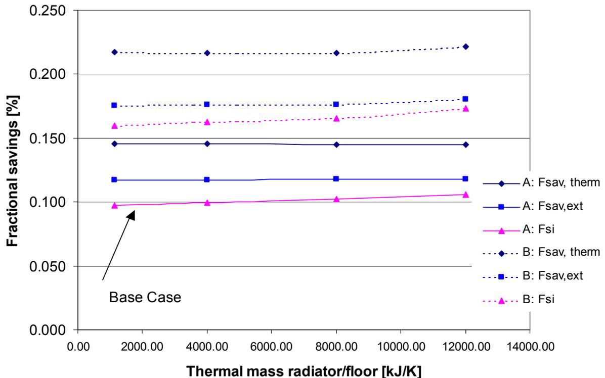
Figure 14: Variation of Radiator Thermal mass. A: 5 m<sup>2</sup> Solar Collector B: 15 m<sup>2</sup> solar collector
