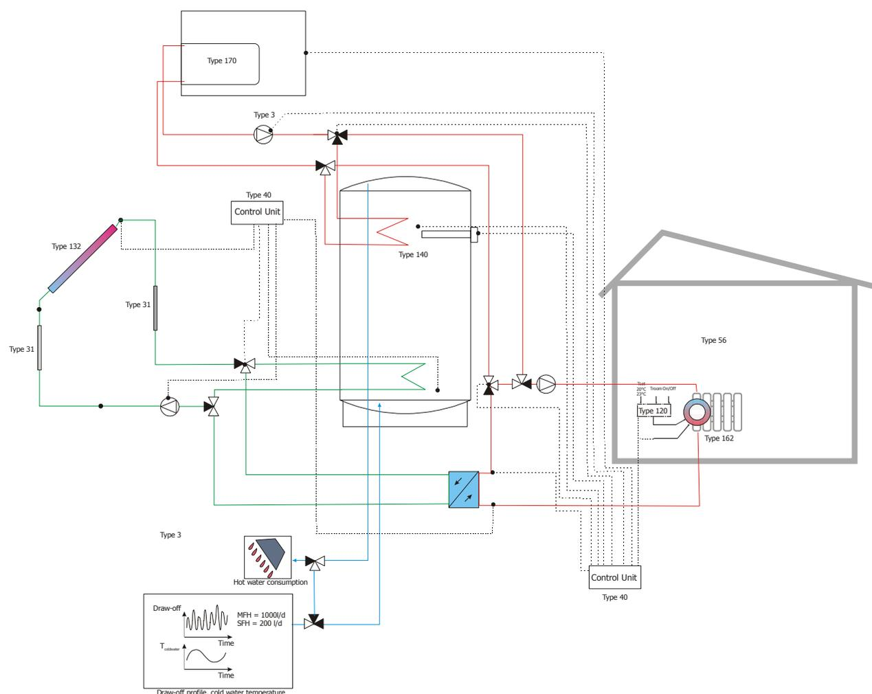
Figure 3: Diagram of System #2 modelled in TRNSYS 14.2
