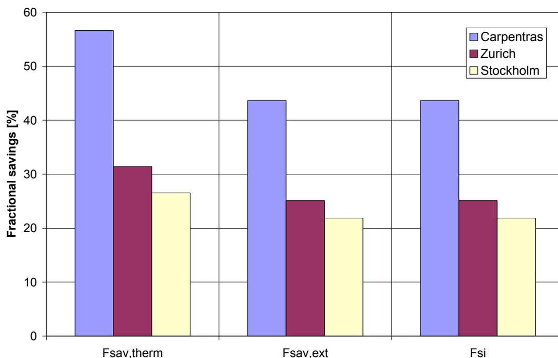
Figure 20. Variation of fractional energy savings for different climates.
