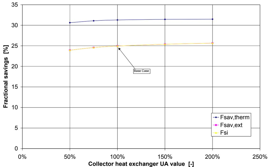
Figure 9. Variation of fractional energy savings with the UA-value of the collector heat exchanger. Parameter values are relative to the values defined for the base case system.
