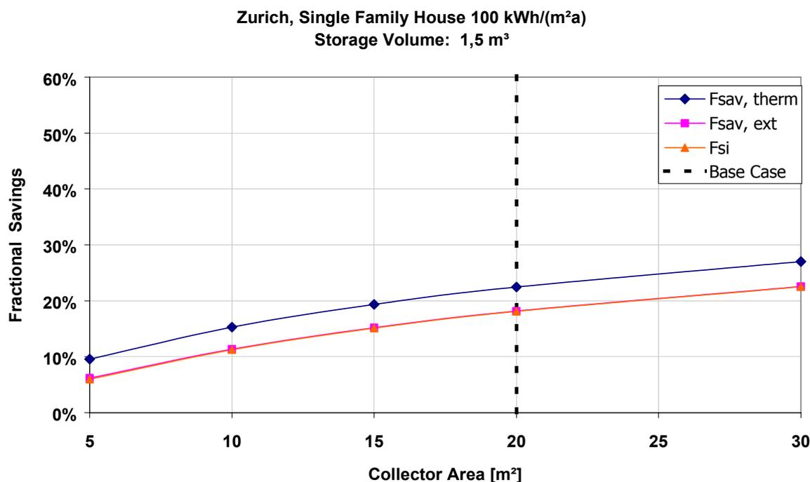
Fig. 10 Variation of fractional energy savings with collector size with fixed store volume of 1.5  $m^3$ . Single-family house 100 kWh/( $m^2a$ ), Zurich.
