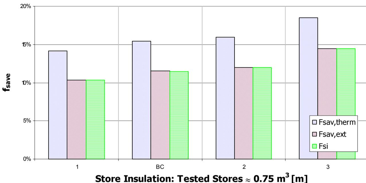
Fig. 21. Variation of fractional energy savings with the heat loss values for stores of about the same volume as the base case store. The heat loss values have been identified from measurements.
