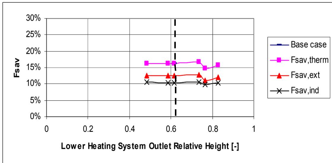
Fig. 15. Variation of fractional energy savings with the position of the lower heating system outlet (flow). Heights are relative heights (=actual height / total height of store)
