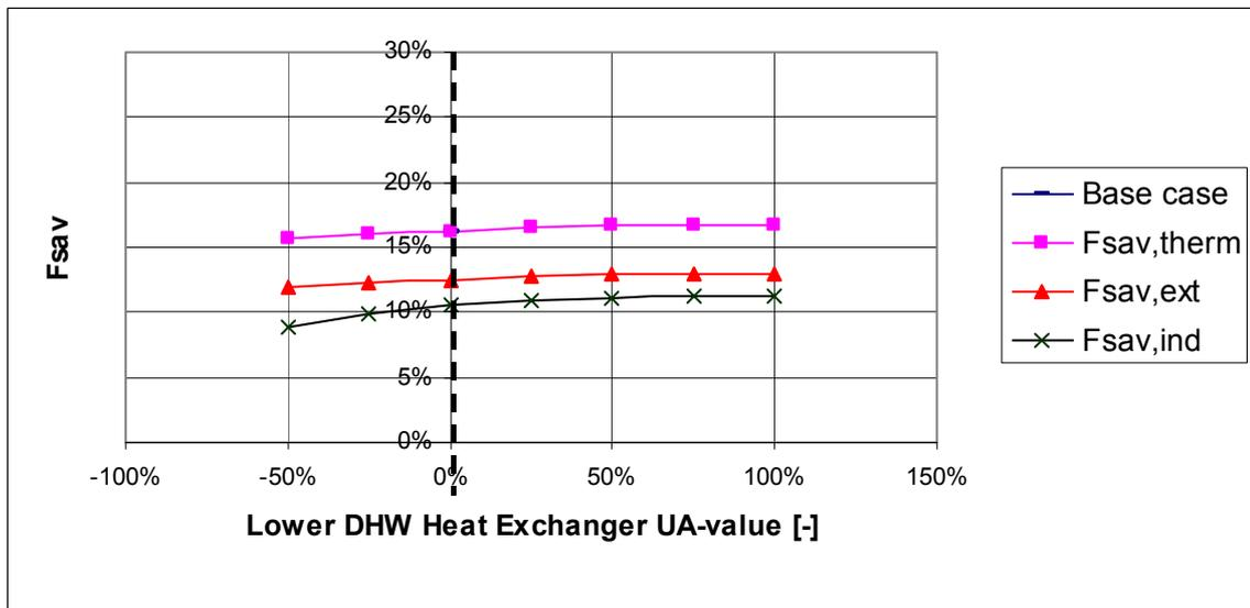
Fig. 19. Variation of fractional energy savings with the UA-value of the lower DHW heat exchanger. Parameter values are relative to that identified from measurements.
