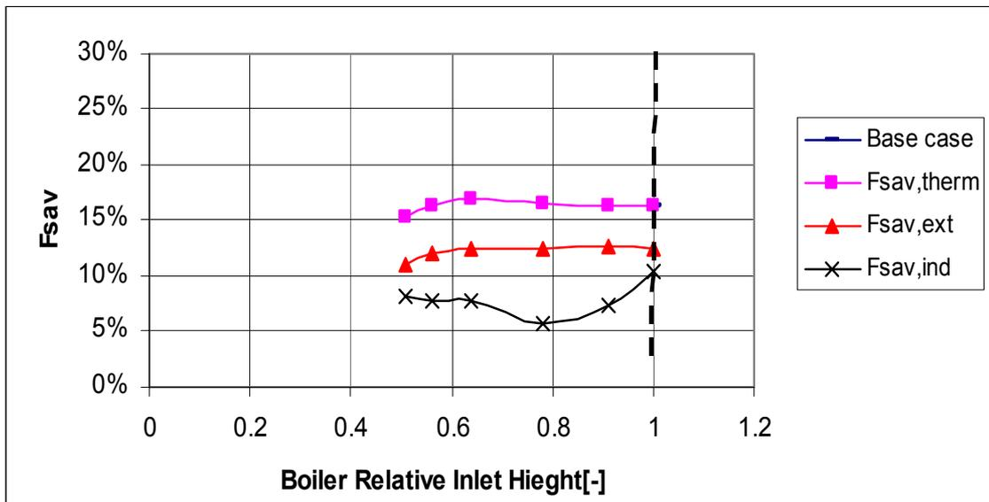
Fig. 11. Variation of fractional energy savings with the position of the boiler inlet. Heights are relative heights (=actual height / total height of store)
