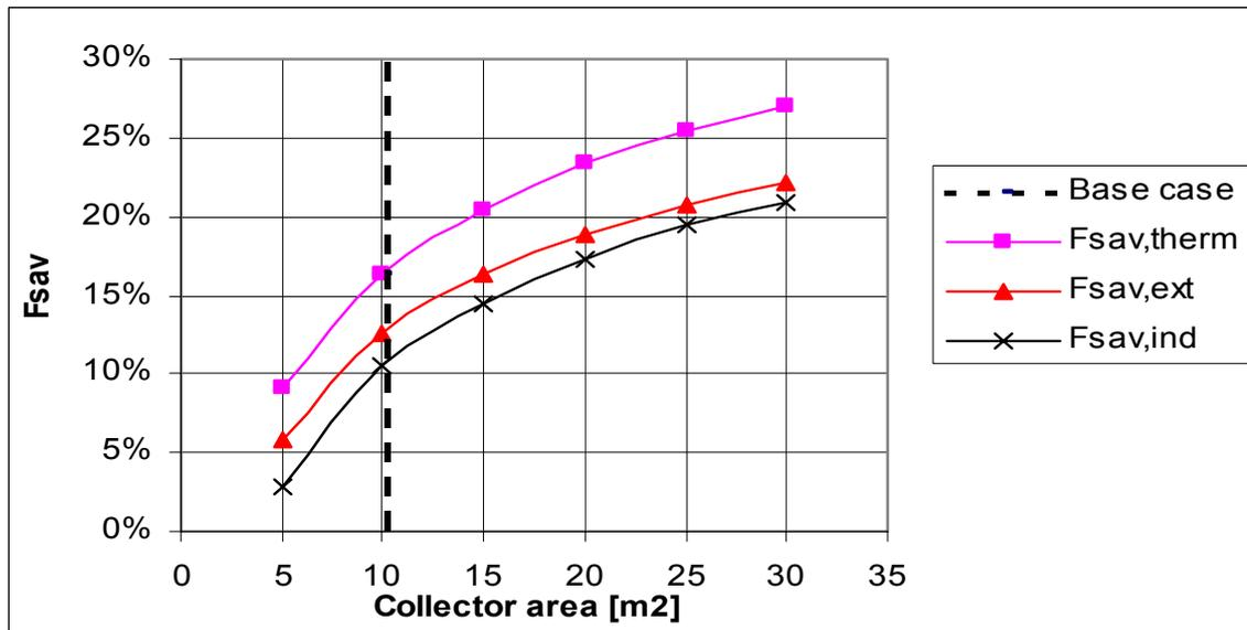
Fig. 2. Variation of fractional energy savings with collector size with fixed store volume of 0.74 m<sup>3</sup>.
