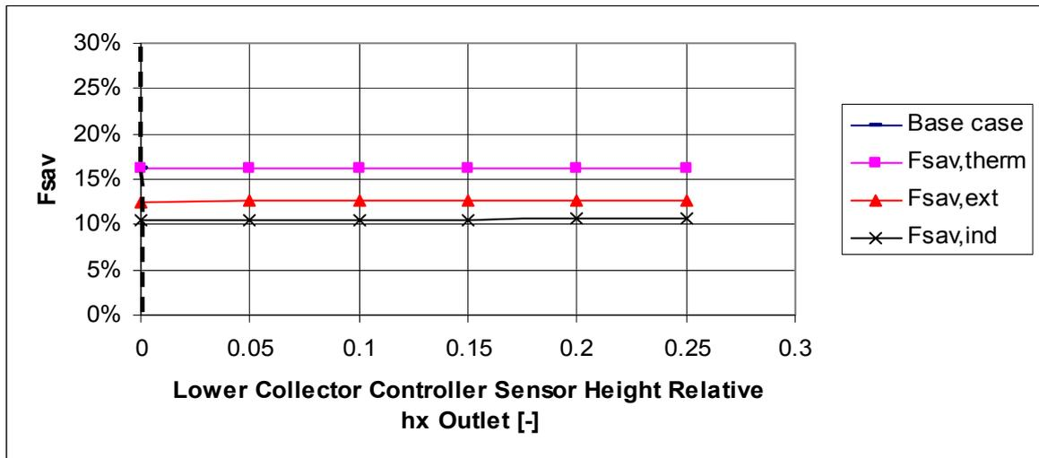
Fig. 27. Variation of fractional energy savings with the collector controller's sensor position.
