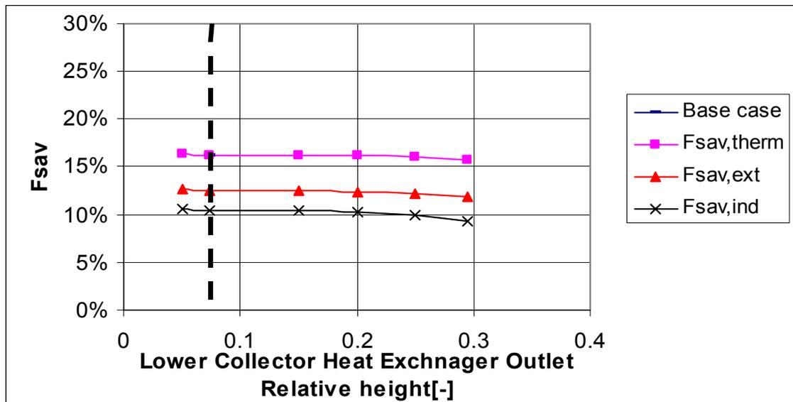
Fig. 8. Variation of fractional energy savings with the position of the lower collector heat exchanger's outlet, with fixed vertical extension of 0.16 for the heat exchanger. Heights are relative heights (=actual height / total height of store)
