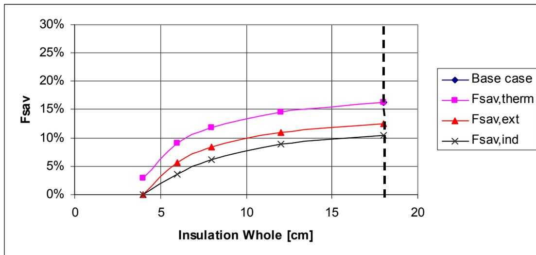
Fig. 24. Variation of fractional energy savings with the thickness of insulation around the whole store.
