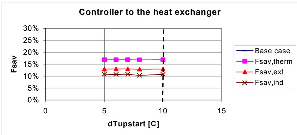
Fig. 29. Variation of fractional energy savings with the upper collector controller's temperature.
