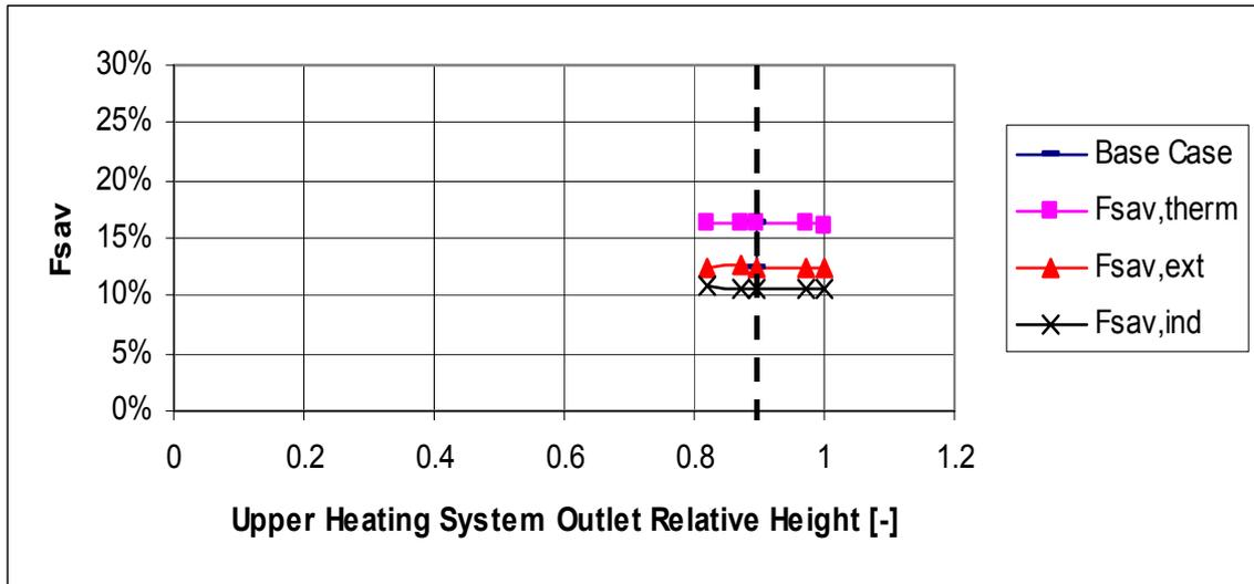
Fig. 16. Variation of fractional energy savings with the position of the upper heating system outlet (flow). Heights are relative heights (=actual height / total height of store)
