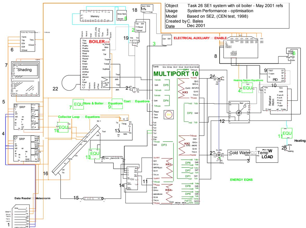
Fig. 1. Modelling of System #12 in PRESIM/TRNSYS. The black numbers are the unit numbers and the green ones the order of the equations sets.
