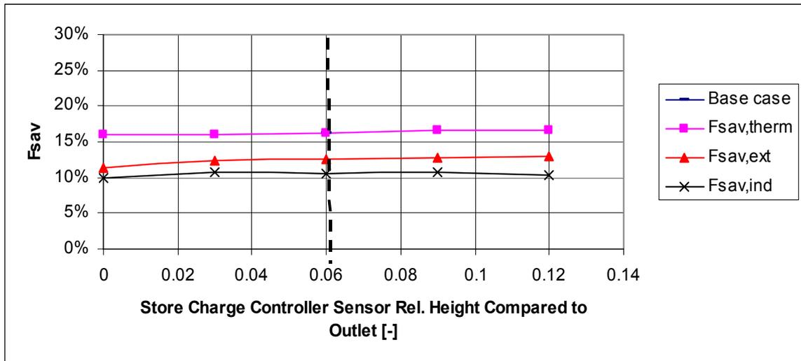
Fig. 26. Variation of fractional energy savings with the store charge controller's sensor position.
