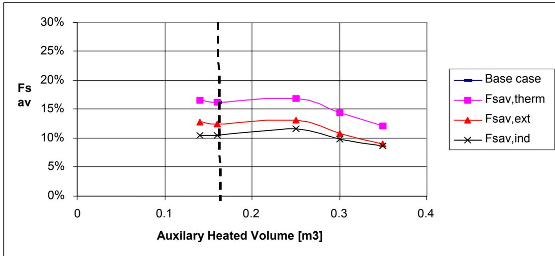
Fig. 13. Variation of fractional energy savings with auxiliary heated volume.
