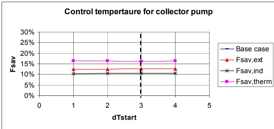
Fig. 30. Variation of fractional energy savings with the control temperature of collector pump.
