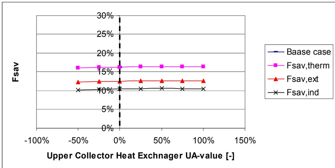
Fig. 18. Variation of fractional energy savings with the UA-value of the upper collector heat exchanger. Parameter values are relative to that identified from measurements.
