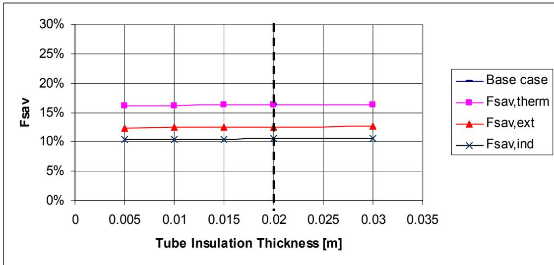
Fig. 31. Variation of fractional energy savings with the insulation thickness round the collector tubing.
