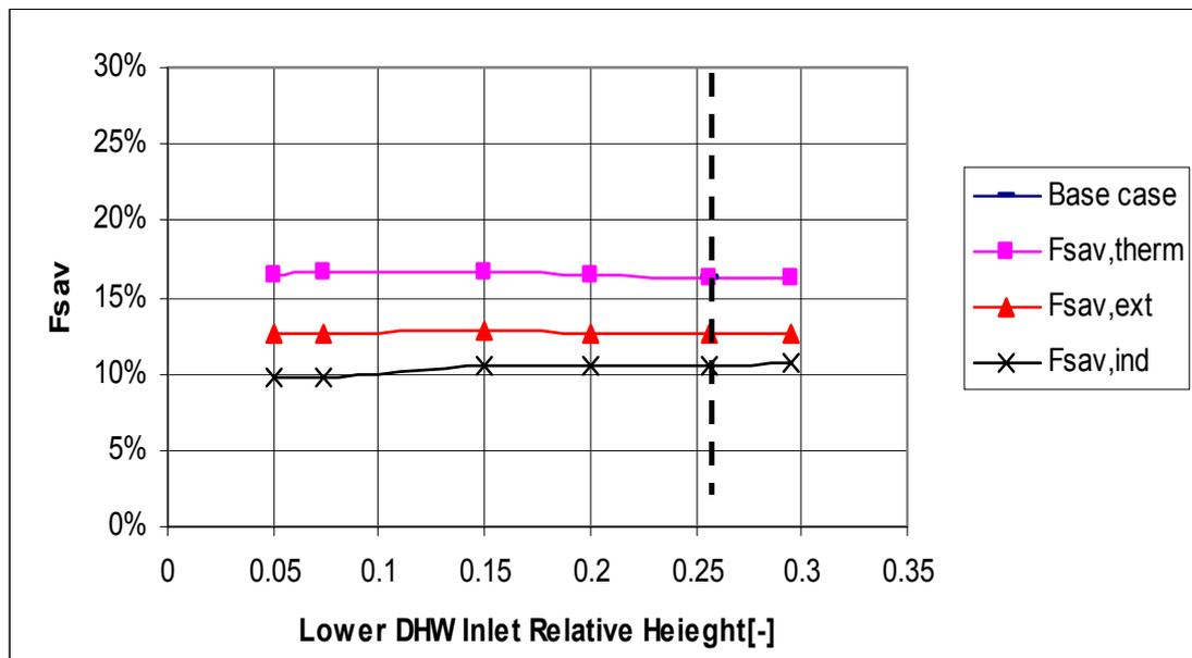
Fig. 9. Variation of fractional energy savings with the position of the lower DHW heat exchanger's inlet, with fixed vertical extension of 0.16 for the heat exchanger. Heights are relative heights (=actual height / total height of store)
