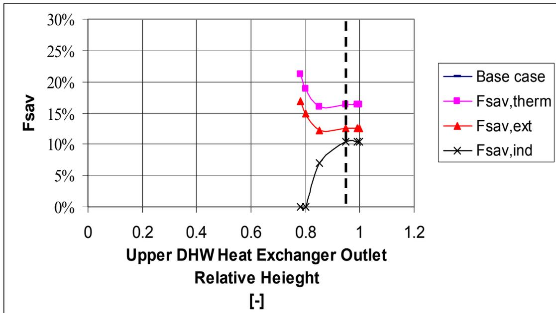
Fig. 10. Variation of fractional energy savings with the position of the upper DHW heat exchanger's outlet, with fixed vertical extension of 0.06 for the heat exchanger. Heights are relative heights (=actual height / total height of store)
