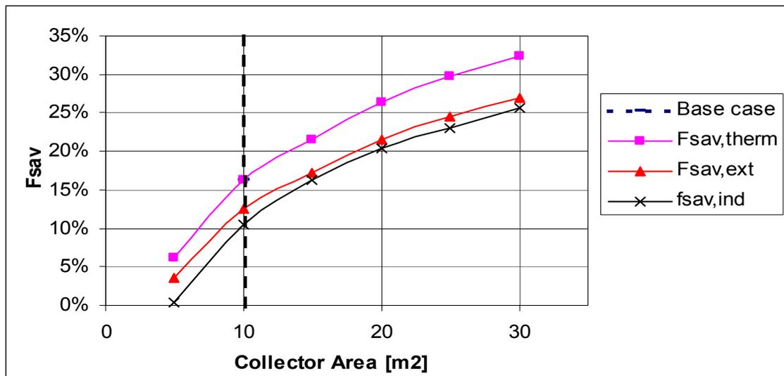
Fig. 3. Variation of fractional energy savings with collector size with fixed specific store volume of 0.074 m<sup>3</sup>/m<sup>2</sup>.
