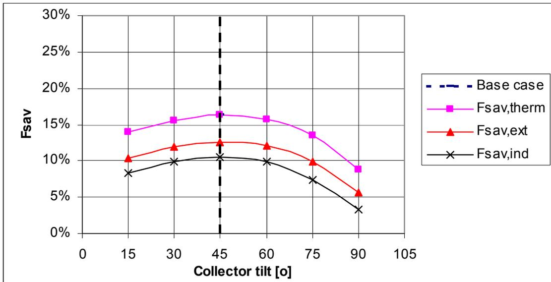
Fig. 6. Variation of fractional energy savings with collector tilt, with fixed azimuth angle of 0°.
