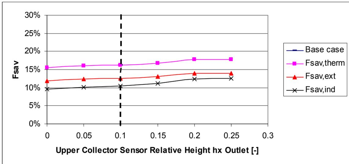
Fig. 28. Variation of fractional energy savings with the upper collector controller's sensor position.
