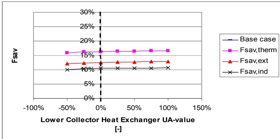
Fig. 17. Variation of fractional energy savings with the UA-value of the lower collector heat exchanger. Parameter values are relative to that identified from measurements.
