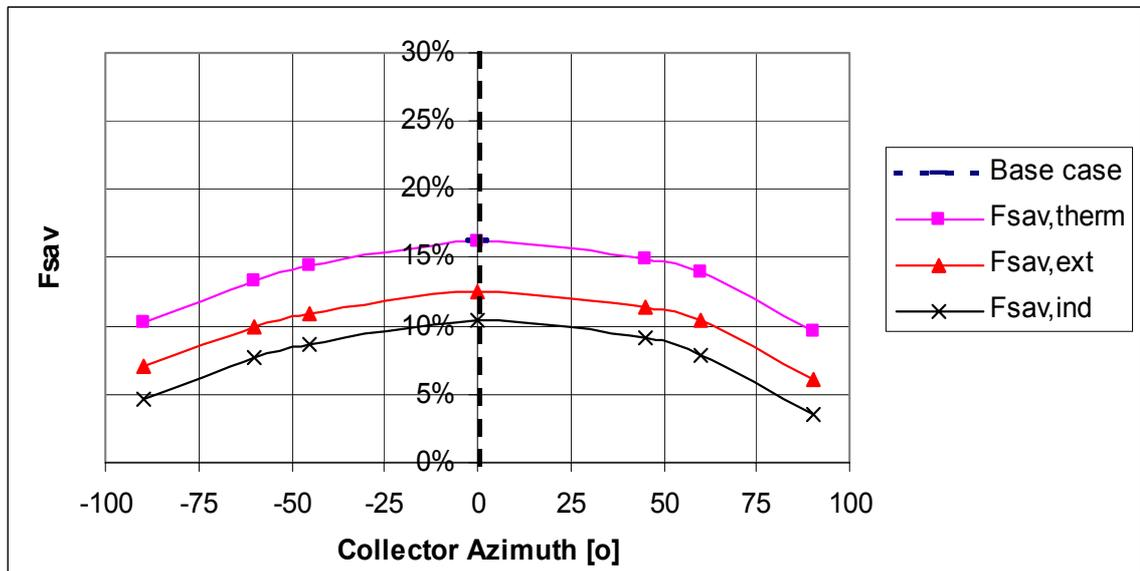
Fig. 5. Variation of fractional energy savings with collector azimuth with fixed tilt angle of 45°.
