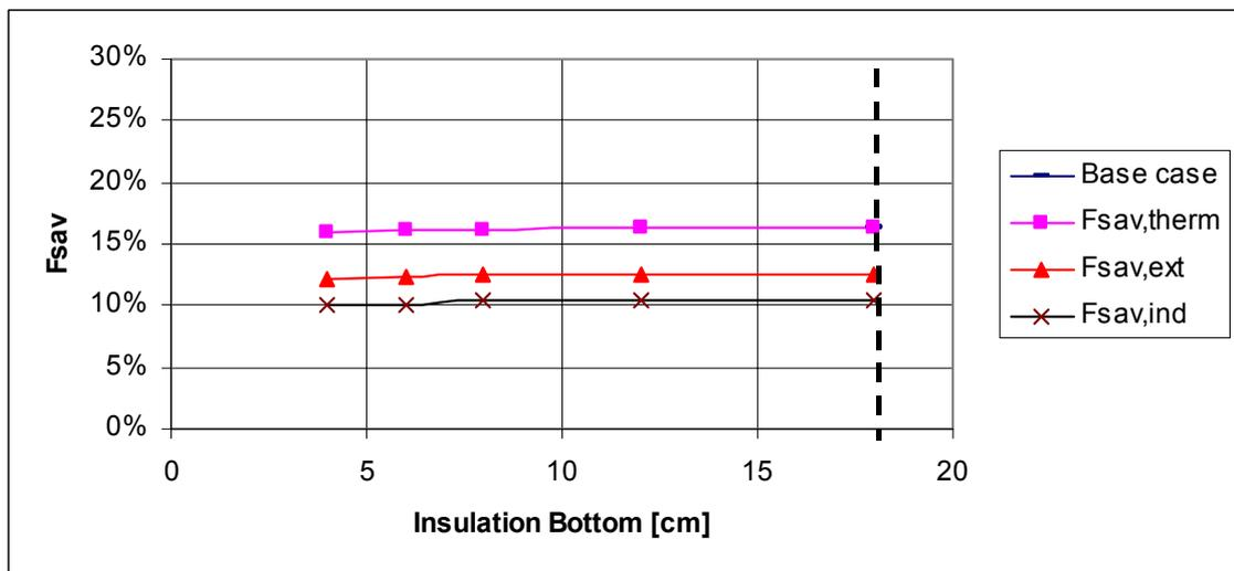
Fig. 23. Variation of fractional energy savings with the thickness of insulation on the bottom of the store.
