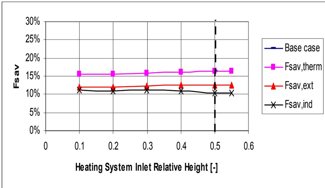
Fig. 14. Variation of fractional energy savings with the position of the heating system inlet (return). Heights are relative heights (=actual height / total height of store)
