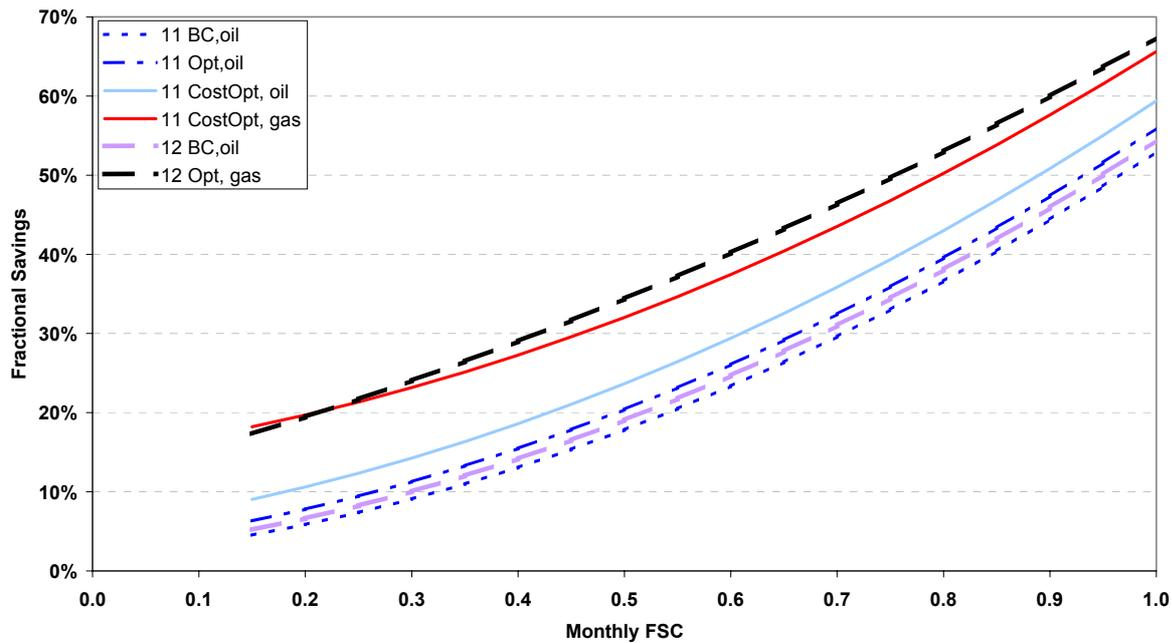
Fig. 32. FSC characteristic for System #12 in the base case simulation model (BC) and optimised version with gas boiler. Characteristics for four version of System #11 are also shown as a comparison.
