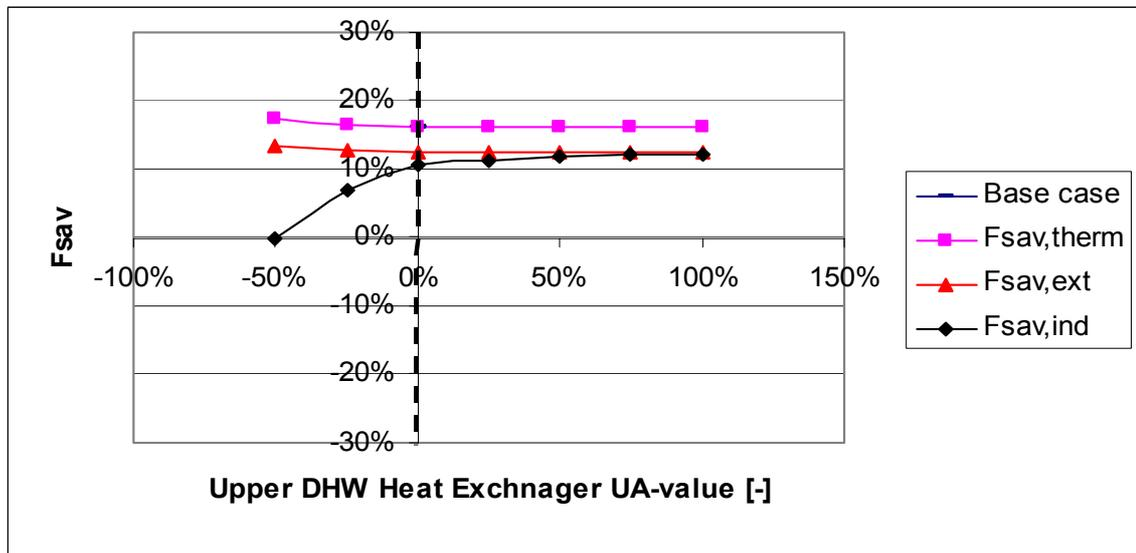
Fig. 20. Variation of fractional energy savings with the UA-value of the upper DHW heat exchanger. Parameter values are relative to that identified from measurements.
