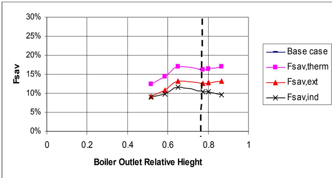
Fig. 12. Variation of fractional energy savings with the position of the boiler outlet. Heights are relative heights (=actual height / total height of store)
