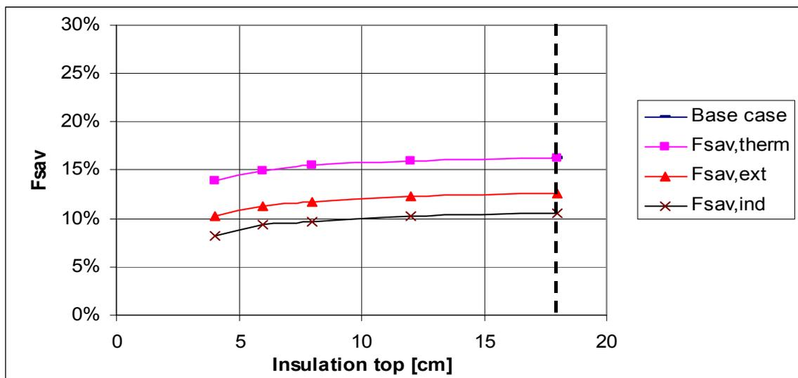
Fig. 21. Variation of fractional energy savings with the thickness of insulation on the top of the store.
