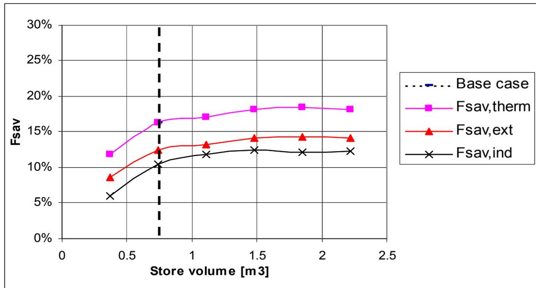
Fig. 4. Variation of fractional energy savings with store volume with fixed collector area of 10 m<sup>2</sup>.
