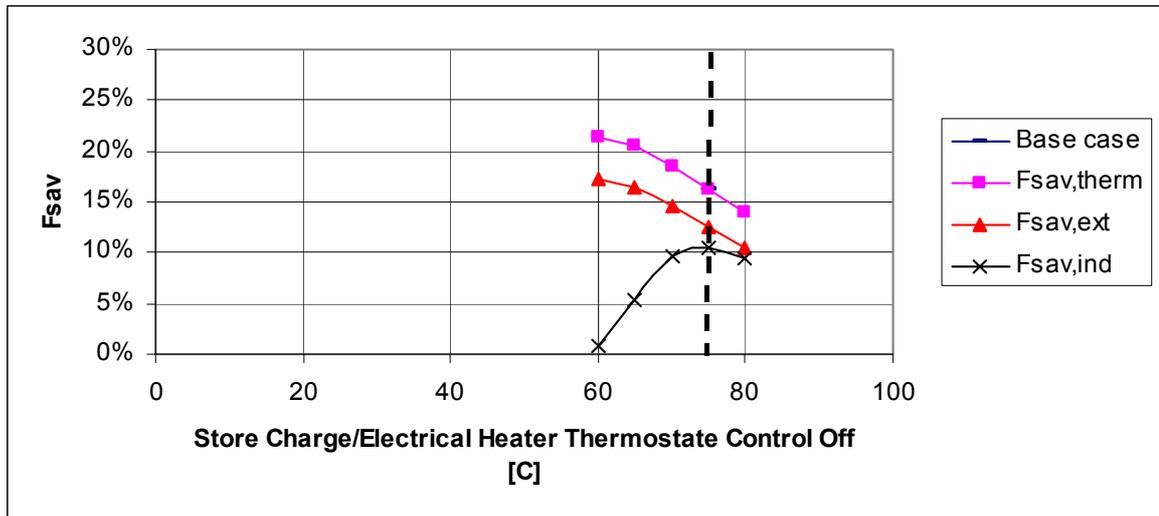
Fig. 25. Variation of fractional energy savings with the store charge controller settings. Values shown are for the charge turn off (upper bound) of the controller.
