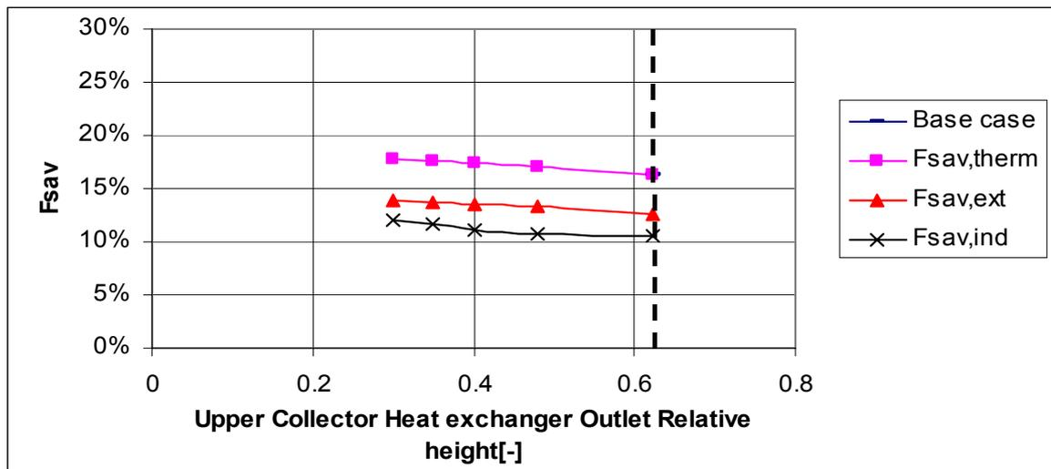
Fig. 7. Variation of fractional energy savings with the position of the upper collector heat exchanger's outlet, with fixed vertical extension of 0.13 for the heat exchanger. Heights are relative heights (=actual height / total height of store)
