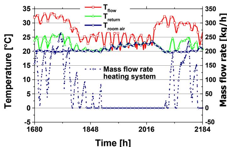
Figure 4: Space heating demand, mass flow rate and temperatures of reference space heating system for a time period of 3 weeks in spring, with radiators and PID controller (thermostatic valve), using DIN 4701 [4] space heating load for the reference SFH 60 in Zurich as the design heating rate
