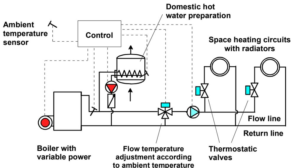
Figure 3: Schematic of the space-heating distribution system of the reference buildings
