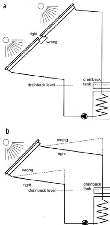
Fig. 1: Examples of correctly, respectively wrongly designed drainback collector loops showing the basic principle of this technology and some of its constraints.
