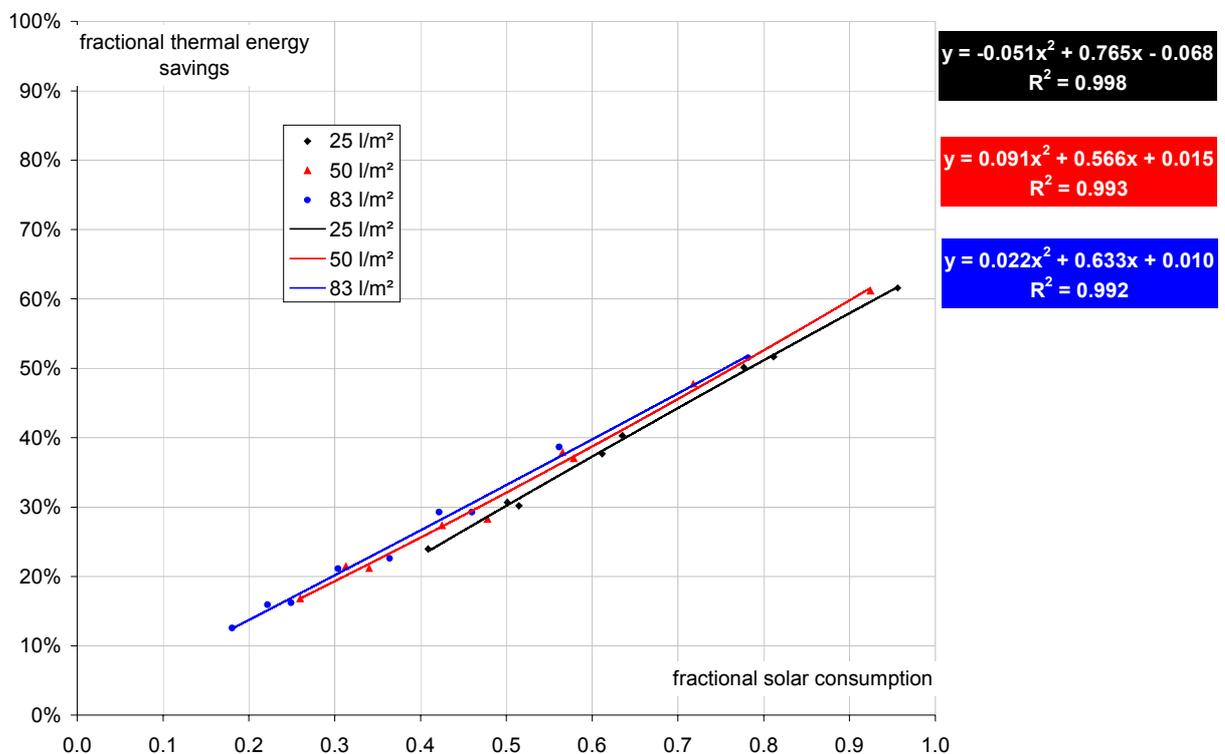
Fig. 6: Fractional thermal energy savings versus fractional solar consumption for System #3a, sorted according to the ratio storage size / collector area
