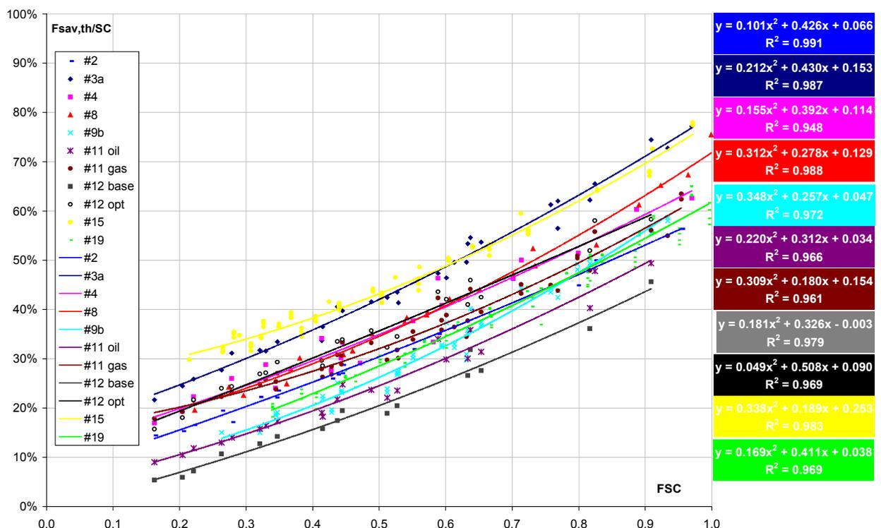
Fig. 7: Fractional thermal energy savings with storage size correction factor, according to fractional solar consumption for systems simulated in task 26
