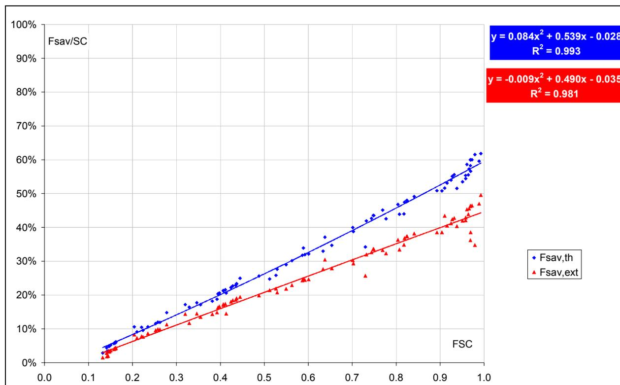
Fig. 17: Fractional energy savings with storage size correction factor, according to fractional solar consumption for System #11 oil (calculations by Chris Bales)
