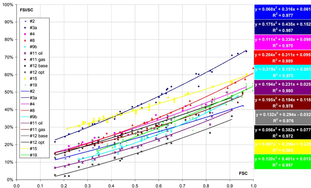
Fig. 10: Fractional solar indicator with storage size correction factor, according to fractional solar consumption for systems simulated in task 26
