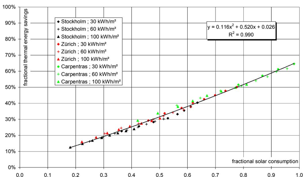
*Fig. 2:* Fractional thermal energy savings versus fractional solar consumption for System #3a, calculated with PSD-MI [2]
