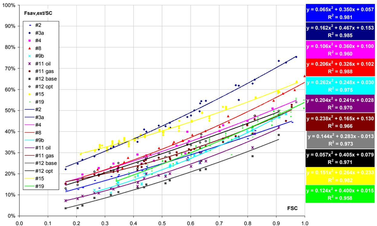
Fig. 9: Extended fractional energy savings with storage size correction factor, according to fractional solar consumption for systems simulated in task 26
