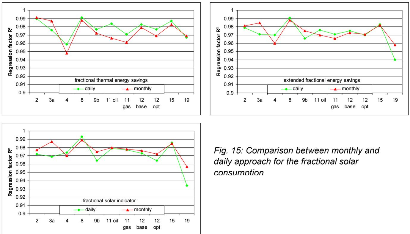
Fig. 15: Comparison between monthly and daily approach for the fractional solar consumption
