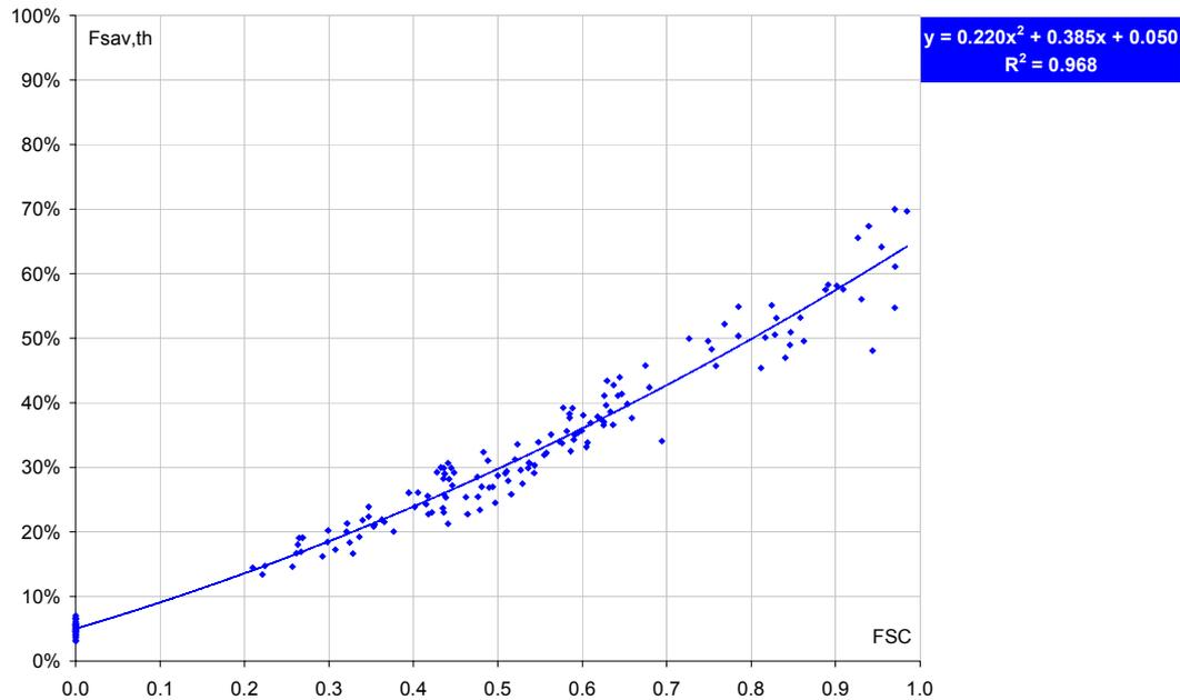
Fig. 18: Fractional energy savings without storage size correction factor, according to fractional solar consumption for System #3a (calculations by Thomas Letz)
