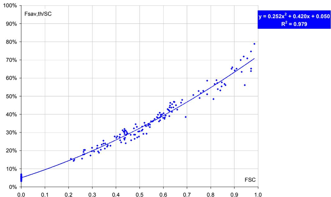
Fig. 19: Fractional energy savings with storage size correction factor, according to fractional solar consumption for System #3a (calculations by Thomas Letz)
