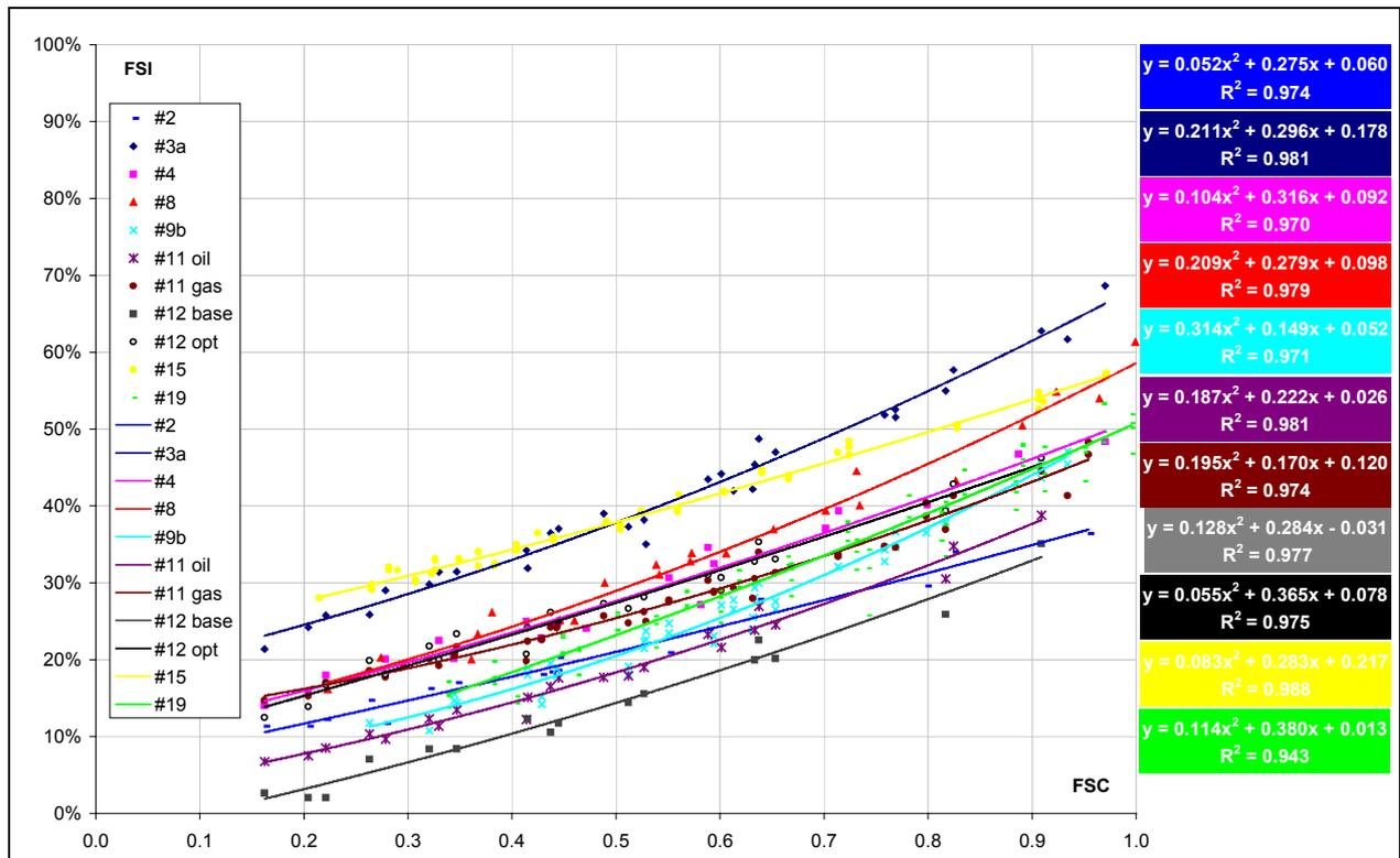
Fig. 5: Fractional solar indicator versus fractional solar consumption for systems simulated in task 26
