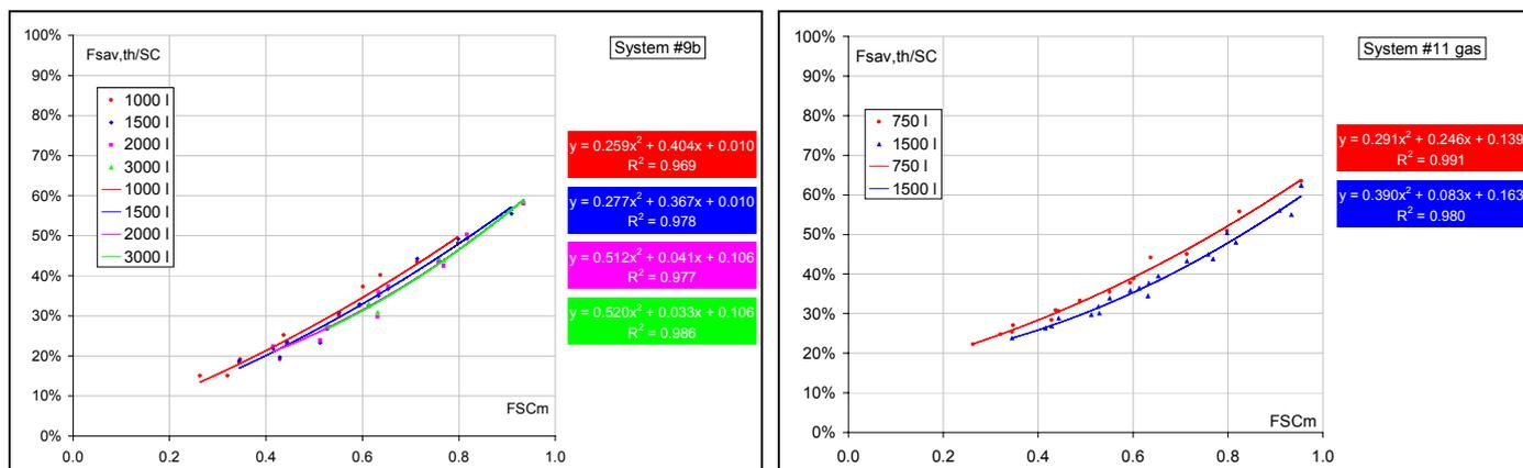
Fig. 11: Fractional thermal energy savings with storage size correction factor, according to fractional solar consumption, sorted out according to storage sizes
