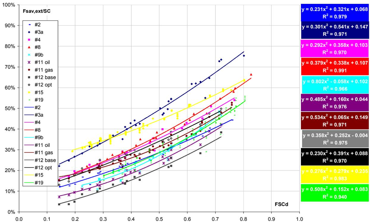
Fig. 13: Extended fractional energy savings with storage size correction factor, versus fractional solar consumption calculated on a daily basis, for systems simulated in task 26
