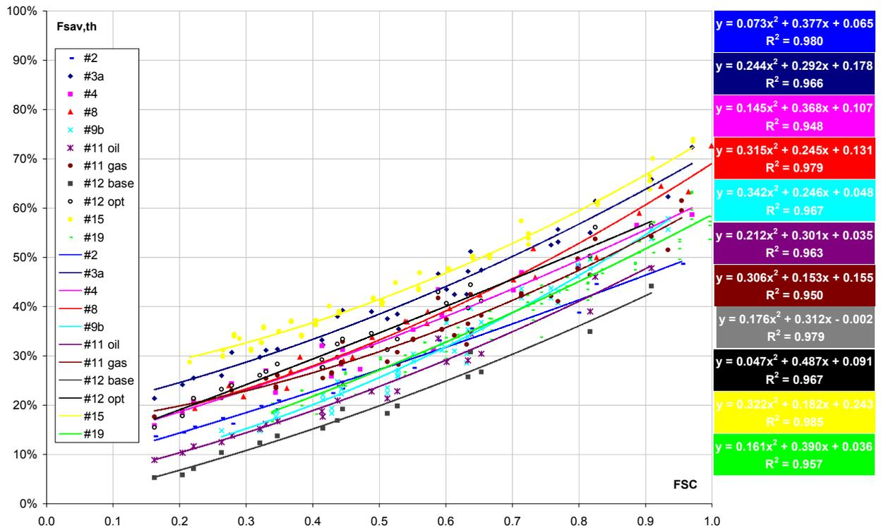
Fig. 3: Fractional thermal energy savings versus fractional solar consumption for systems simulated in task 26
