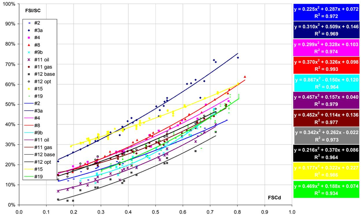
Fig. 14: Fractional solar indicator with storage size correction factor, according to fractional solar consumption calculated on a daily basis, for systems simulated in task 26
