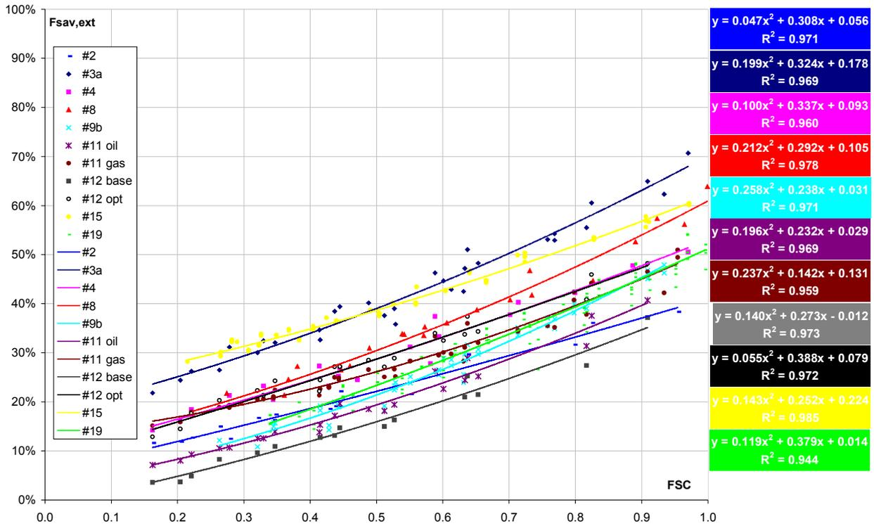
Fig. 4: Extended fractional energy savings versus fractional solar consumption for systems simulated in task 26
