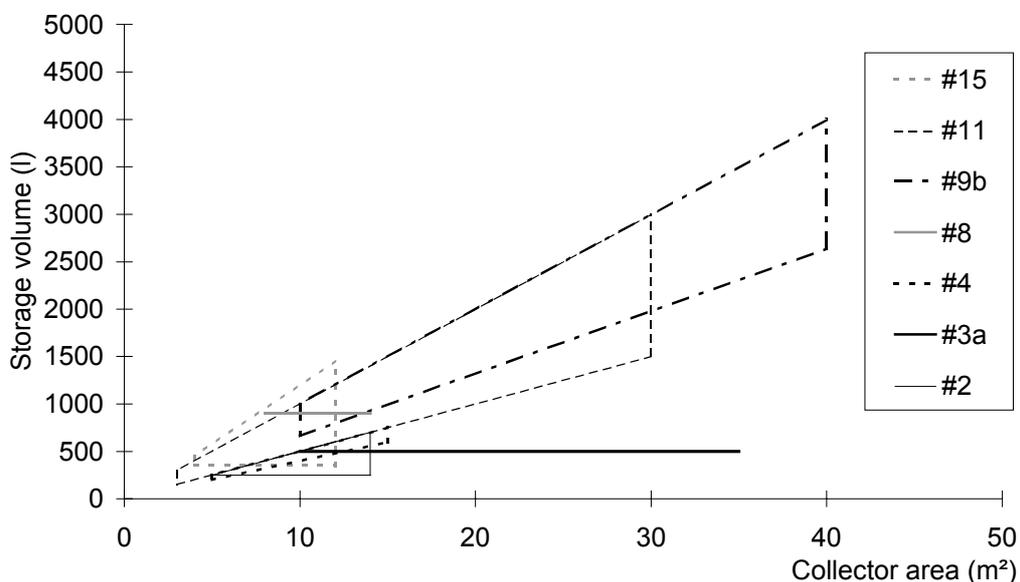
Fig. 21: Example of size diagram of combisystems (numbers refer to the generic systems)
