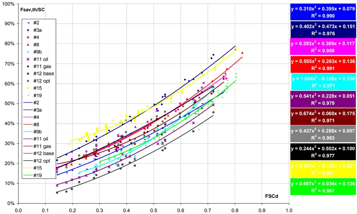
Fig. 12: Fractional thermal energy savings with storage size correction factor, versus fractional solar consumption calculated on a daily basis, for systems simulated in task 26
