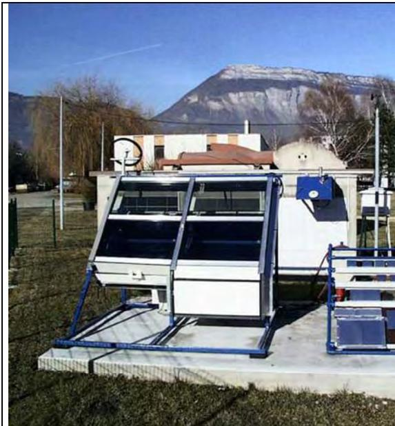
Fig. 6: View of the test box for outdoor exposure and meteorological instruments at CSTB
