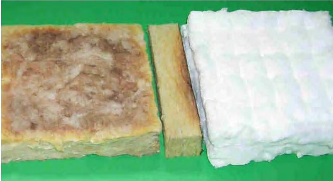
Fig. 4: Photo of different insulation materials based on mineral wool after treatment in a small test solar collector at stagnation temperatures for 24 hours (left and middle: top view and cross section of a mineral wool containing phenolic resin; right: binder-free wool)
