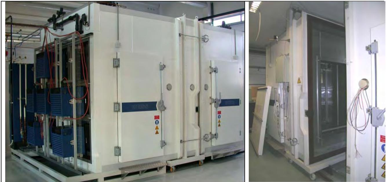
Figure 5.4: Climatic chamber and sample holder, which allows the installation of samples with dimensions of more than 1.8 m times 1.5 m.
