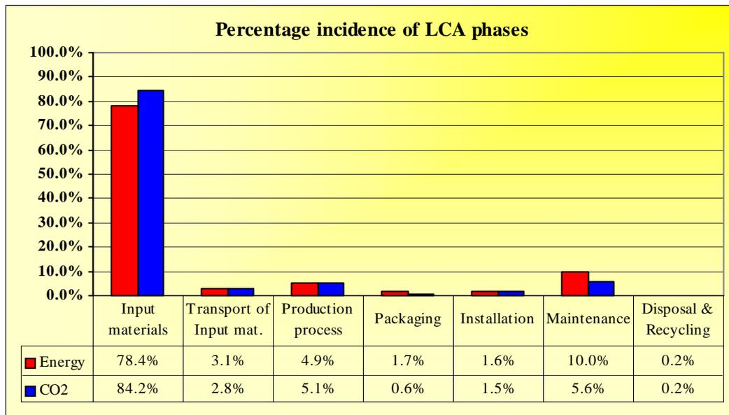
**Fig. 5: Percentage incidence of LCA phases on global energy consumption and CO<sub>2</sub> emission**
