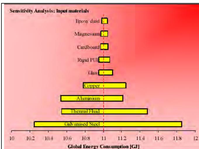
Fig. 5: Sensitivity analysis of the global energy consumption due to input materials
