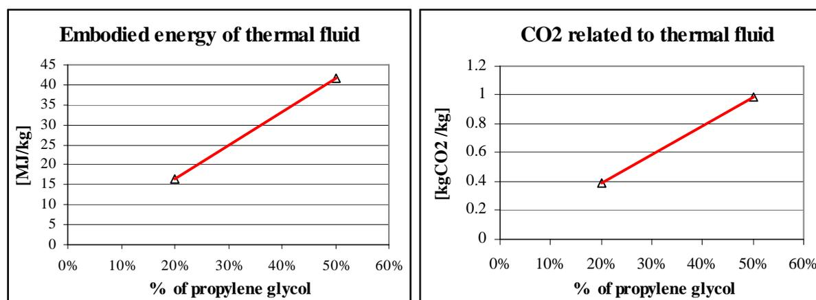
**Fig. 2: Embodied energy and CO<sub>2</sub> emissions for variable percentages of glycol in the thermal fluid**
