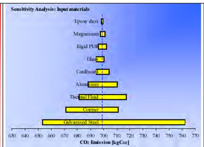
Fig. 6: Sensitivity analysis of the CO<sub>2</sub> emissions due to input materials
