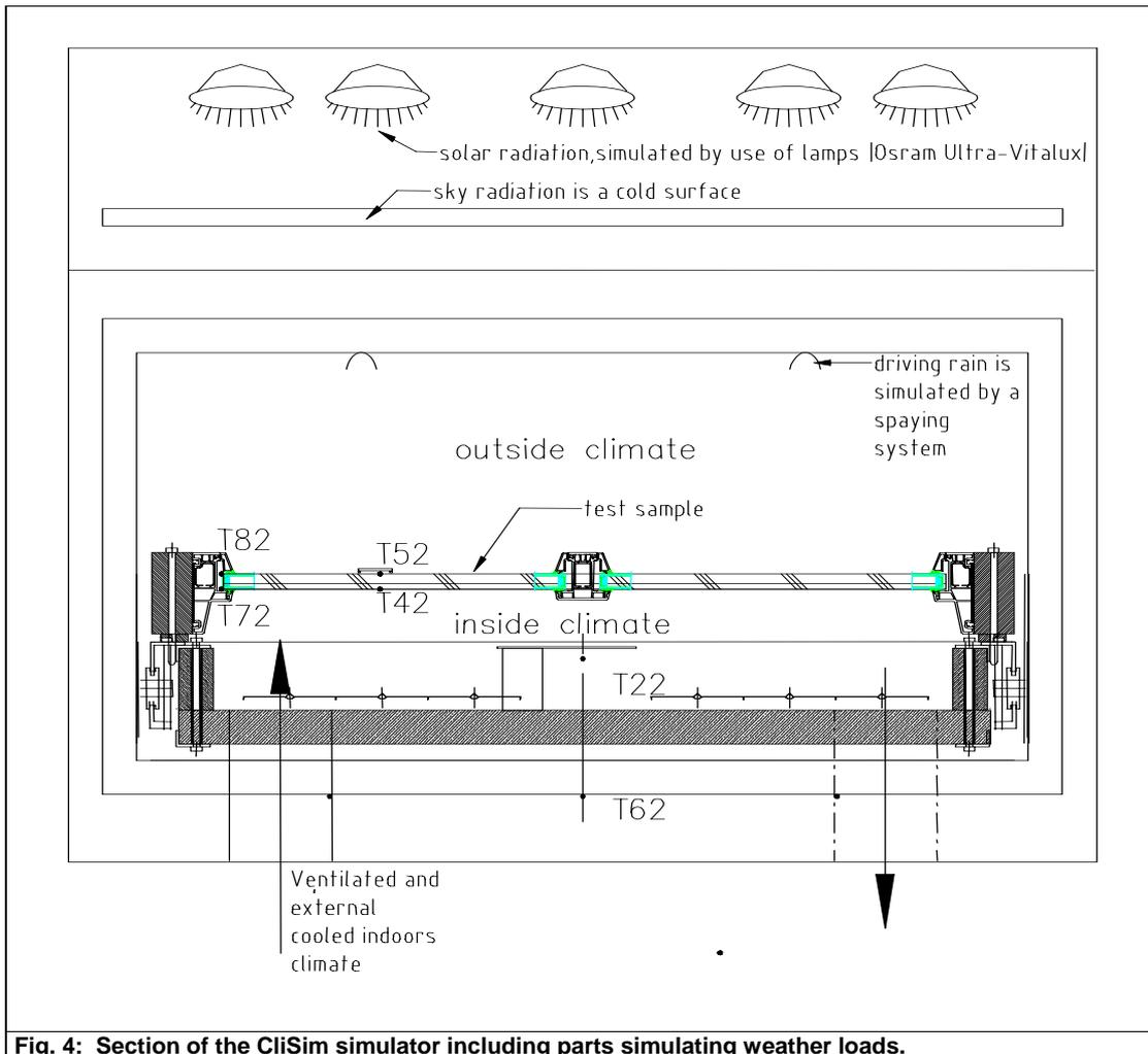
Fig. 4: Section of the Clisim simulator including parts simulating weather loads.
