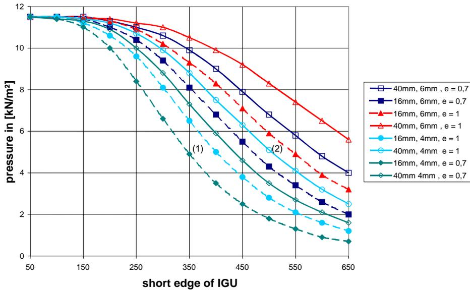
Fig. 32: Internal pressure for aspect ratio of 0,7 and 1,0, thickness of glass panes of 4 mm and 6 mm and for interpane separation of 16 mm and 40 mm
