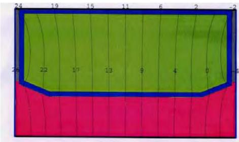
**Fig. 2: Isotherms for an aluminum spacer with a conductivity of  $160 \text{ W/m K}$ . Thickness of metal  $0.36 \text{ mm}$**
