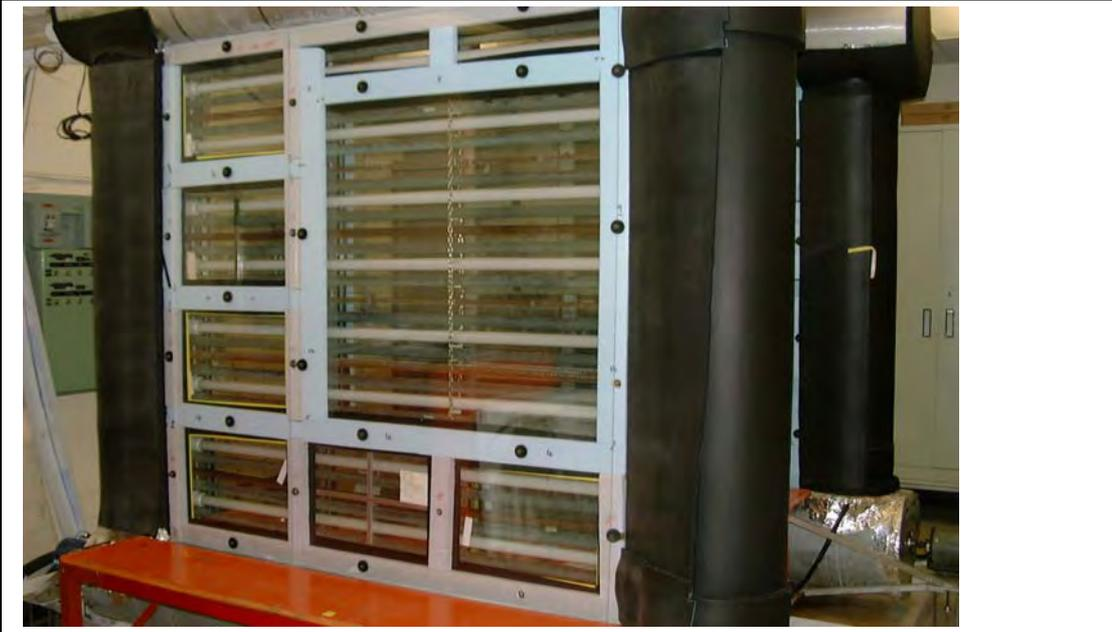
Fig. 8: IG units mounted in the weather cycling apparatus.
