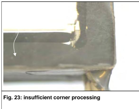
**Fig. 23: insufficient corner processing**
