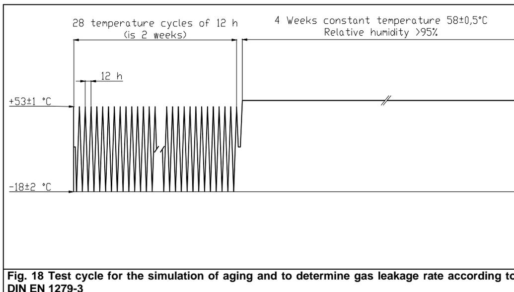
**Fig. 18 Test cycle for the simulation of aging and to determine gas leakage rate according to DIN EN 1279-3**
