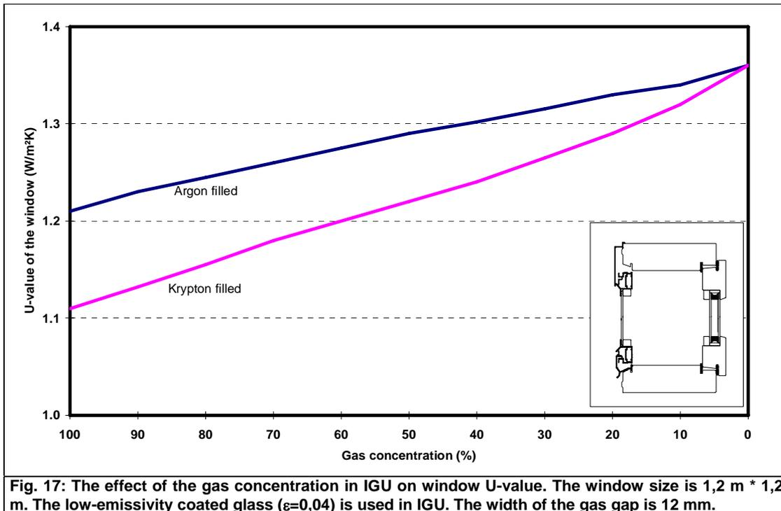
Fig. 17: The effect of the gas concentration in IGU on window U-value. The window size is 1,2 m \* 1,2 m. The low-emissivity coated glass ( $\epsilon=0,04$ ) is used in IGU. The width of the gas gap is 12 mm.
