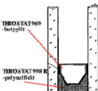
Fig. 1: Systems of insulating glass units (double-sealed box spacer)
