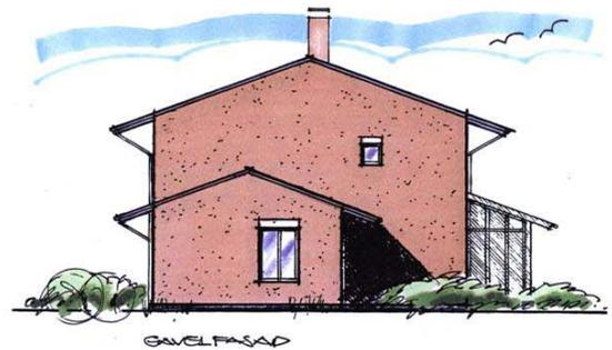
The windows are triple-glazed with low emission coating and gas in between. The windows facing south and west have also an extra coating in order to decrease the solar radiation through the windows. The g-value is 0,34. The U-value for the windows, including frames, varies between 0,9 and 1,0 W/(m<sup>2</sup>·K) depending on window size. The glassed area corresponds to approx. 20% of the floor area.
