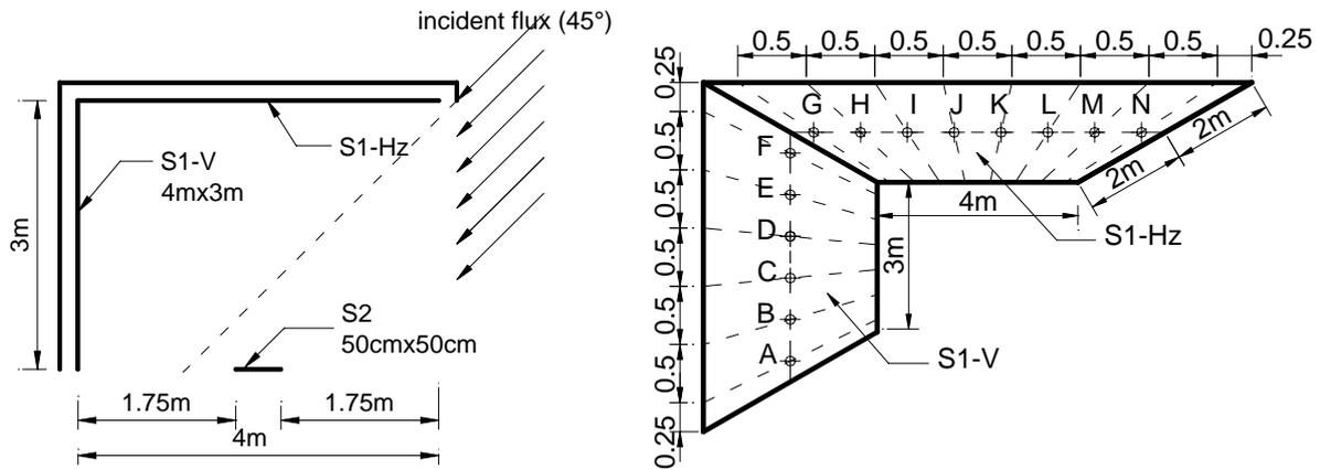
Figure 16: Test case description for 50cmx50cm diffusing surface (S2) and measurement points' position
