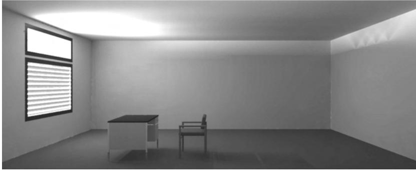
Fig. 6. Photo-realistic visualization of room illuminated by standard venetian blinds in the lower façade area and a light redirecting glass in the upper façade area.
