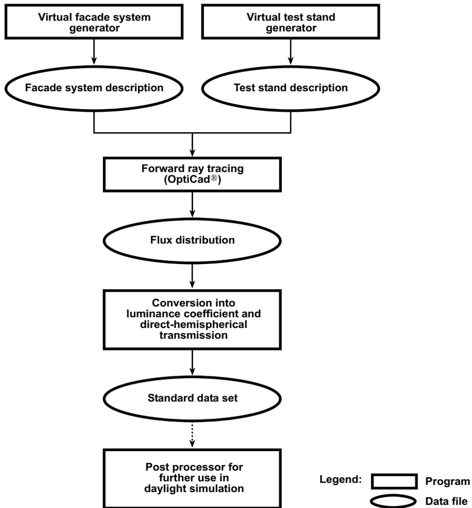
Fig. 5. Flowchart illustrating the program interaction and dataflow of the FHG-IBP numerical goniophotometer environment.
