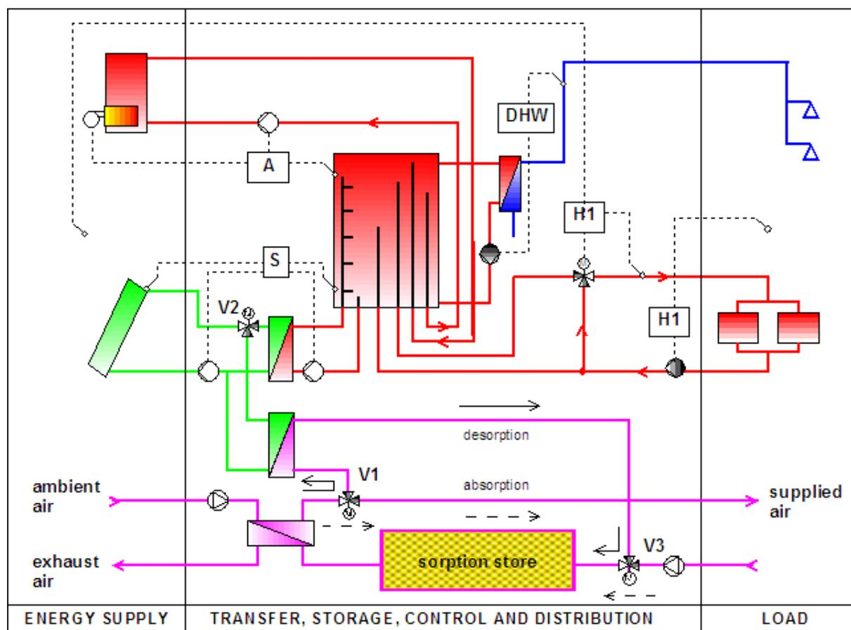
Figure 1. Principal configuration of the monosorp system.
