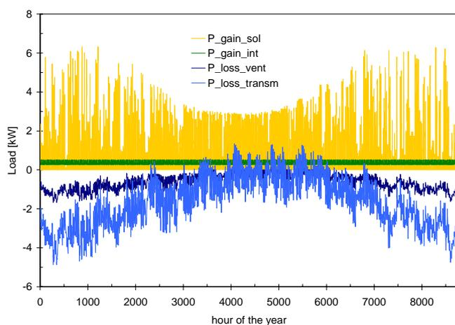
Figure 2.1: Solar gains  $P_{gain,sol}$ , internal gains  $P_{gain,int}$ , ventilation losses  $P_{loss,vent}$  and transmission losses  $P_{loss,transm}$  in the course of the year
