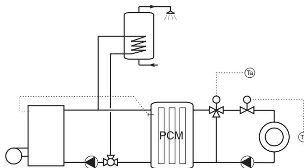
*Figure 2.11: Hydraulic scheme of system G2b – gas boiler, water tank with integrated PCM modules*
