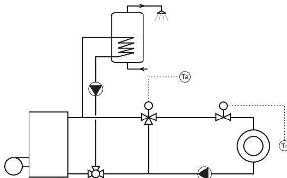
Figure 2.7: Hydraulic scheme of system G1b – system with mixture control
