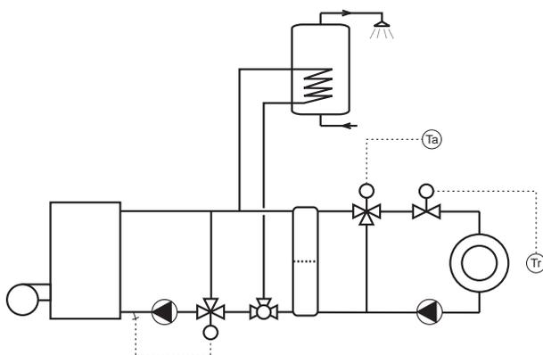
Figure 2.9: Hydraulic scheme of system P1 – system with mixture control, hydraulic switch, return temperature control
