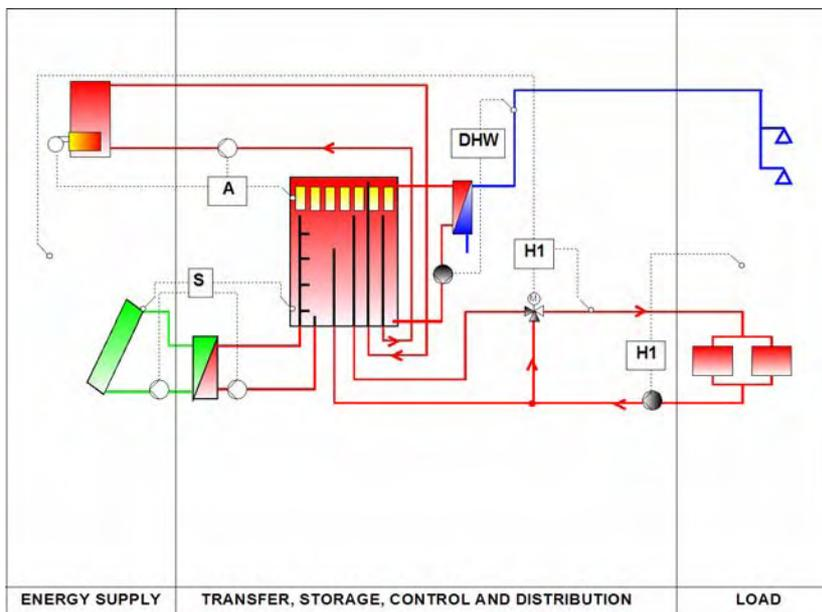
Figure 5: Simulated solar combisystem of University of Lleida, Spain
