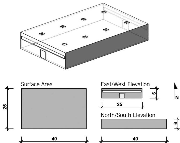
Fig. 7 Dimensions of the reference building.
