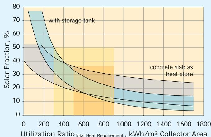
Nomograms are useful because they help to decide whether it is necessary to use a water filled storage tank or if it makes sense to use the thermal mass of the concrete floor slab as heat storage. The advantage of using the concrete floor slab is that the costs for a (often times large) storage tank can be saved.
