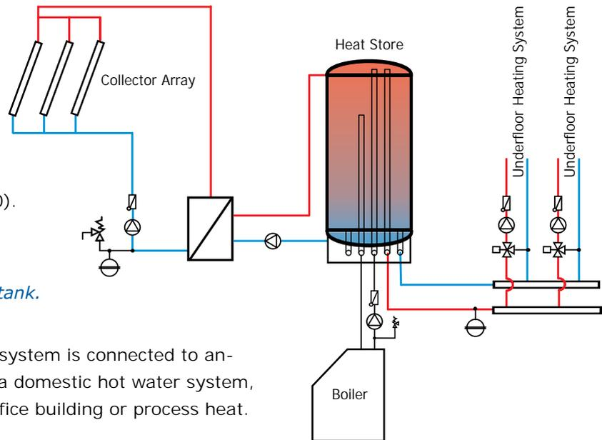
Fig. 10 System concept with storage tank.
