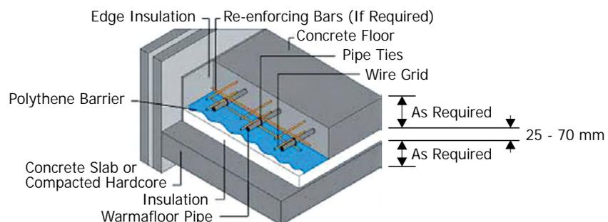
Fig. 6 Influence of depth of piping in an underfloor heating system.
