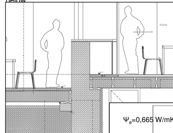
Construction detail and thermal conductivity image of the connection. The effect of the higher ground temperatures from the extra insulation is clearly visible.
