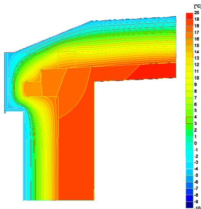
Reduction of thermal bridge at the eaves ( $\psi = 0.04 \text{ W/mK}$ ).
