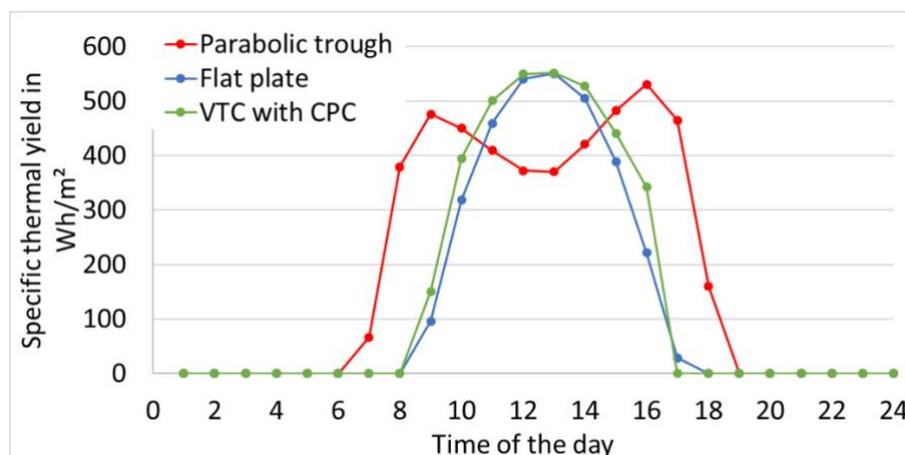
**Figure 1: Profile on 14<sup>th</sup> September for the climate of Potsdam, Germany (Meteonorm 7.3), at 75 °C and a North-South axis for the parabolic trough collector.**
