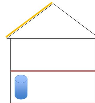
120 m<sup>3</sup> thermal activation of building mass (27/20°C), 1m<sup>3</sup> water tank (95/30°C)
